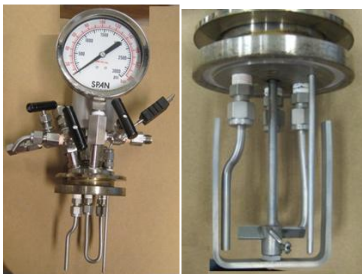
Figure 5-1 Reactor Head and Internals
