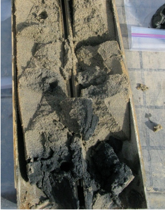
Figure 11 - Staining at approximately 9 mbgs at MW-402
