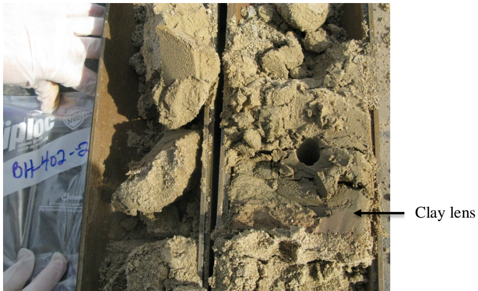
Figure 4 – Core sample showing sand with clay lens from the target area in BH-402 at 7.9 mbgs
