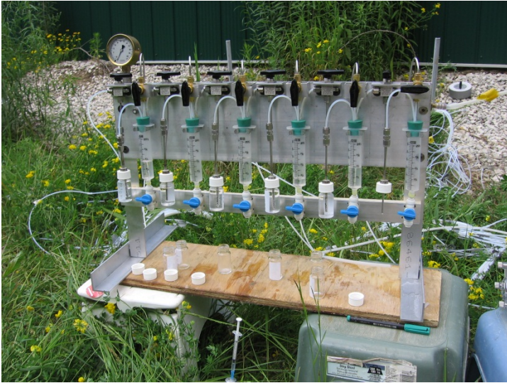
Figure 37 - Sampling manifold for volatile sampling. Photo: J.G. Freitas
