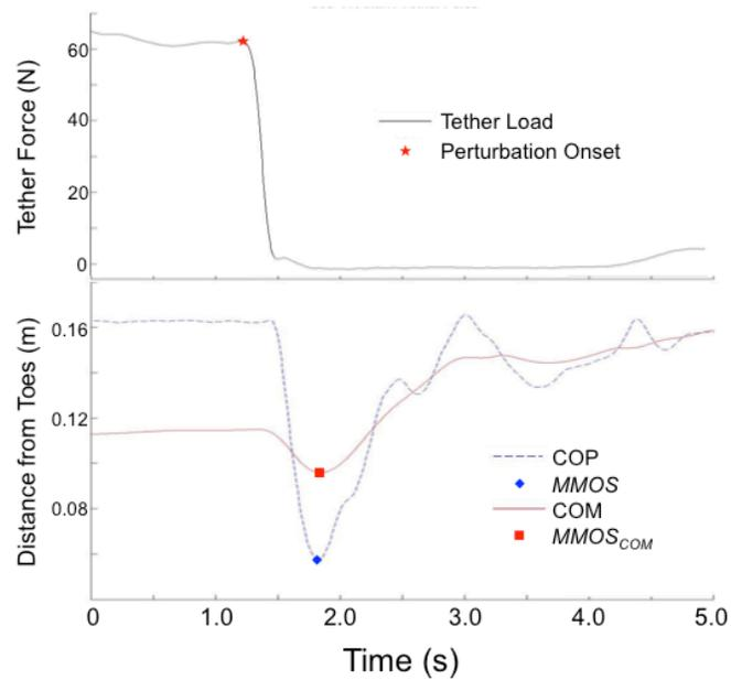
**Figure 3-2: Representative force profile recorded from the tether load cell over the entire course of one trial on the commercial carpet, indicating the moment of perturbation onset (upper); Representative COP and COM displacement profiles over the entire course of one trial, plotted as distance from the toes (lower)**
