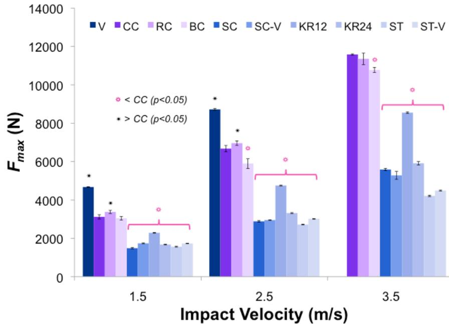
**Figure 2-6: Mean (SD) peak forces applied following impacts to the back of the headform at each impact velocity across all flooring conditions**
