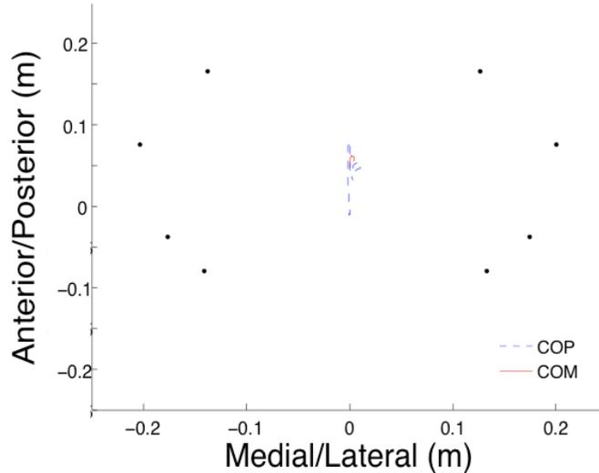
**Figure 3-3: Representative anterior/posterior versus medial/lateral displacement profiles for the COP and COM following perturbation onset for one trial on the commercial carpet (with respect to the centre of the force plate); black dots indicate location of (from top to bottom) markers on the hallux, fifth metatarsal, lateral malleolus, and heel of the left and right feet**
