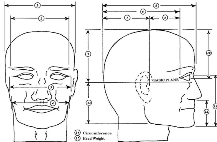
**Figure 1-6: Pictorial description of the anthropometric dimensioning used for NOCSAE headforms (adapted from NOCSAE, 2009)**
