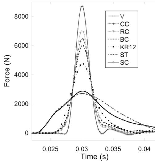
**Figure 2-2: Representative force versus time profiles from 2.5 m/s impacts onto a subset of the floor conditions tested.**
