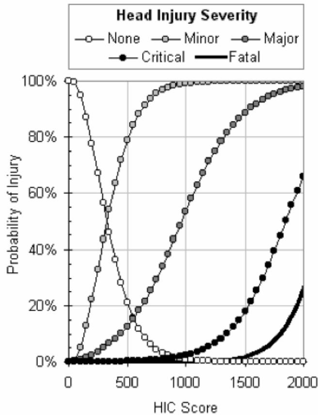
**Figure 1-5: Expanded Prasad-Mertz curves demonstrating the relationship between HIC score and probability of head injury (from Shorten and Himmelsbach, 2003); At a HIC score of 1000, the probability of suffering no injury is reduced to zero, while the probability of a fatal injury becomes non-zero**
