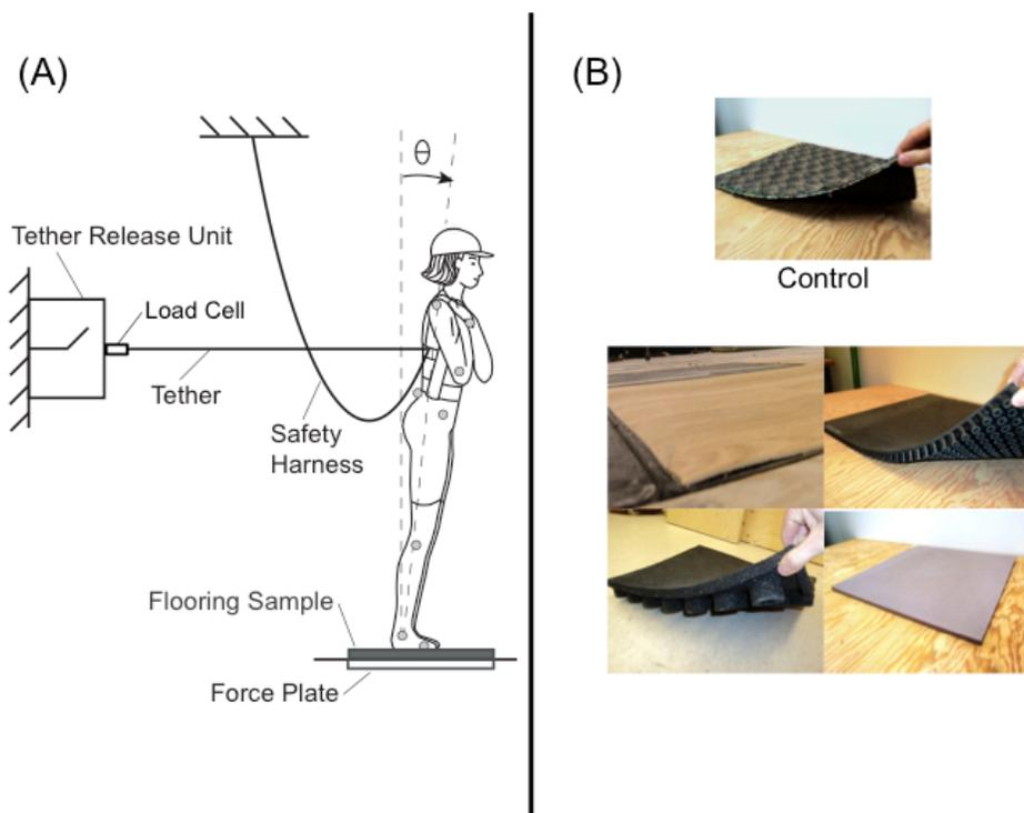
**Figure 3-1: A) Schematic of the experimental setup to used for the tether-release experiment; B) Pictures of the floor conditions tested: Top – Commercial Carpet (CC - control); additional floors (clockwise from top left): Vinyl (V), SmartCell (SC-V), 12 mm Kradal (KR), and SofTile (ST-V); note that SmartCell and Vinyl were tested with vinyl overlay.**
