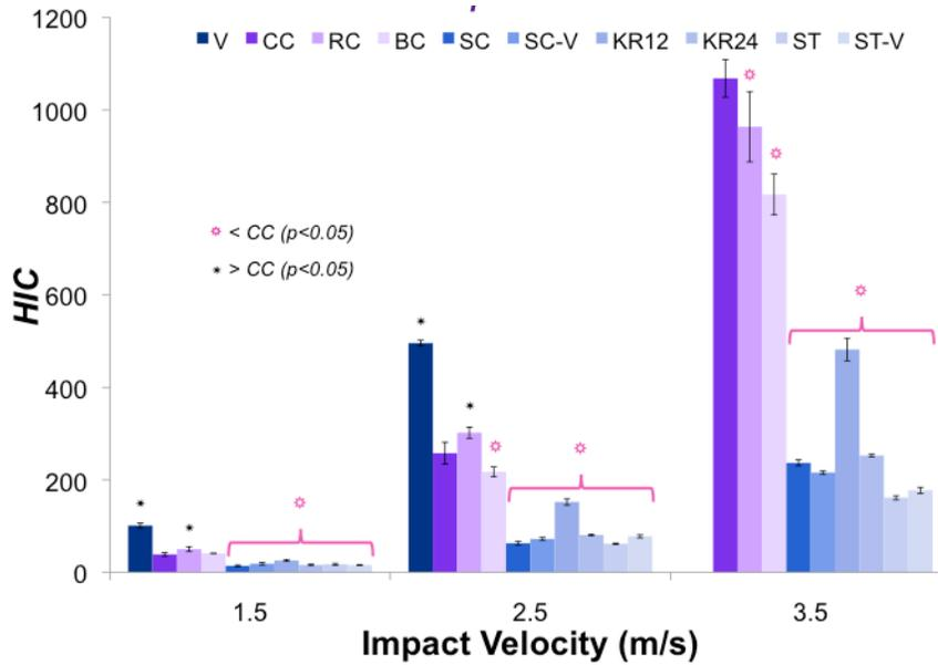
**Figure 2-5: Mean (SD) Head Injury Criterion (HIC) scores for impacts onto the back of the headform at each impact velocity across all flooring conditions**
