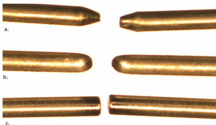
Figure 10. Magnified image of NTD tips (10x). a. House tapered (HT) NTD. b. SGE tapered NTD. c. Blunt (B) tip NTD.
