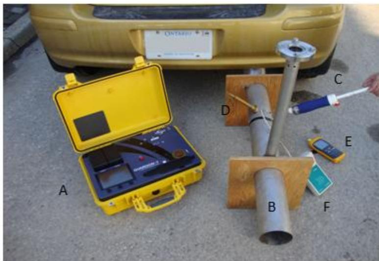
Figure 18. On-site sampling of gasoline exhaust. (A) GUARDION-7, (B) custom exhaust sampling device, (C) NTD vacuum syringe, (D) SPME sampler, (E) thermometer, (F) flow meter.
