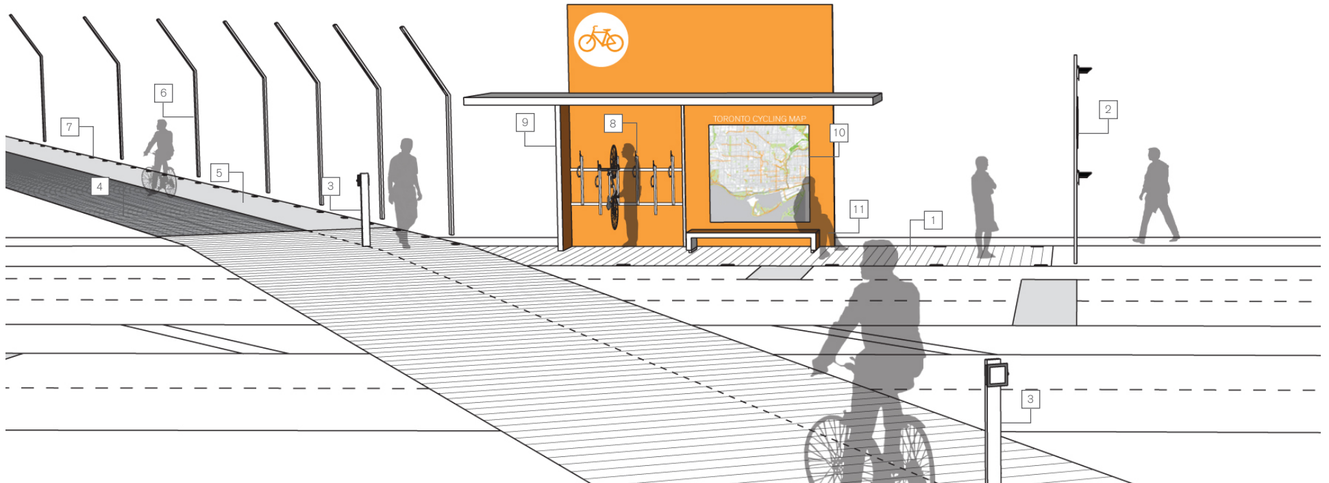
Fig.4.35 Push button crossing stands and path patterns gives cyclists and pedestrians the right-of-way over vehicular traffic. Hub H1 allows cyclists to pair with existing transit networks by providing sheltered parking.
