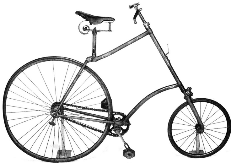
Fig.2.4 The Humber 'Safety' bicycle of 1884 had nearly all of the features of a contemporary machine: low-mount profile, rear wheel drive powered by a chain, and inflatable rubber tires.
