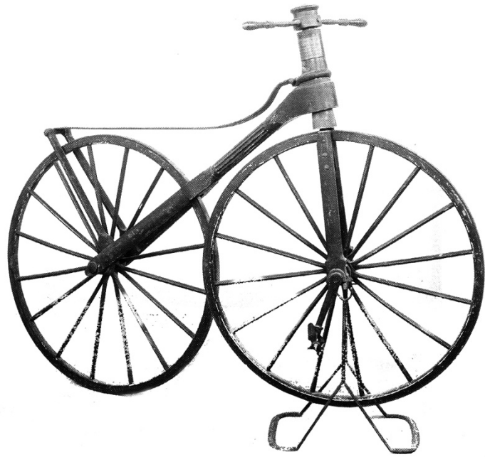
Fig.2.3 A wooden prototype of a diagonal-frame bicycle during the 'Boneshaker' era of the 1860's.
