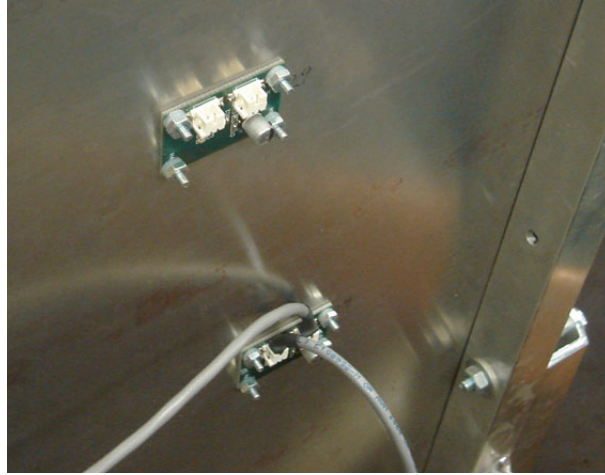
Figure 3.18: Detail view of microphone PCBs from the rear of the array
