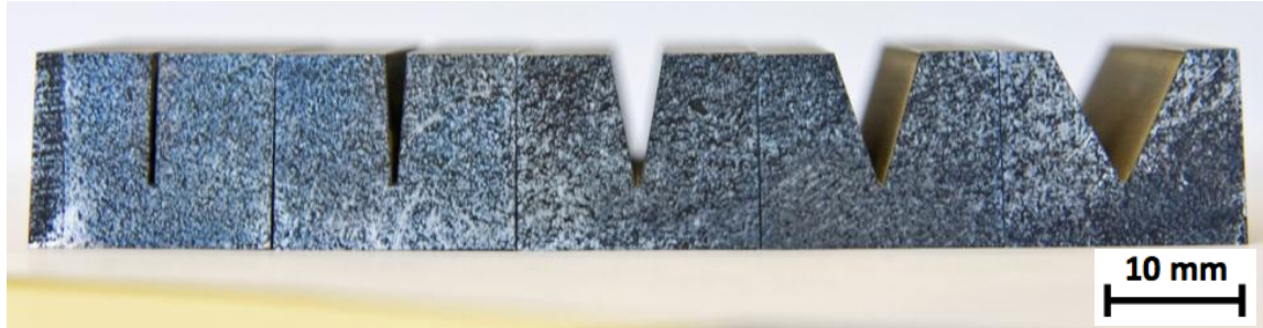
Figure 3.1: Coupons (15 mm x 12 mm x 9 mm) with notches of 8mm depth and widths of (from left to right) 0.25, 1, 3, 5, and 8 mm.
