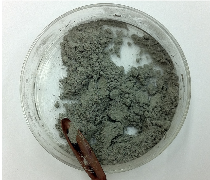
Figure 3.4: Filler metal powder mixtures after wet ball-milling, resulting in a fully-mixed combination of base and filler metal powders.
