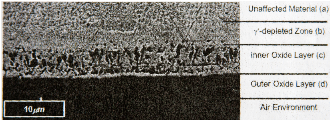
Figure 2.6: Micrograph of the distinct oxide regions observed on GTD111 after oxidation at 982°C for 312 hours [19].
