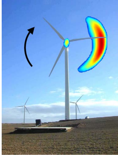
Figure 2.17: Beam map of a 58 m diameter turbine shown with a 12 dB range from Oerlemans [41]
