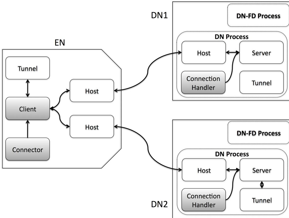
Figure 4.2: Accorriem Components: Modified Modules shown in Gray
