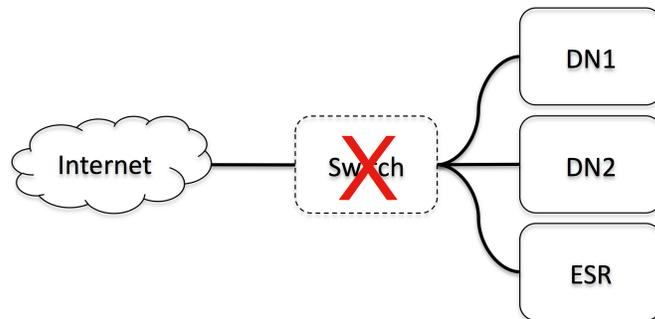
b) Failure of an intermediate network device, disconnecting all DNs
