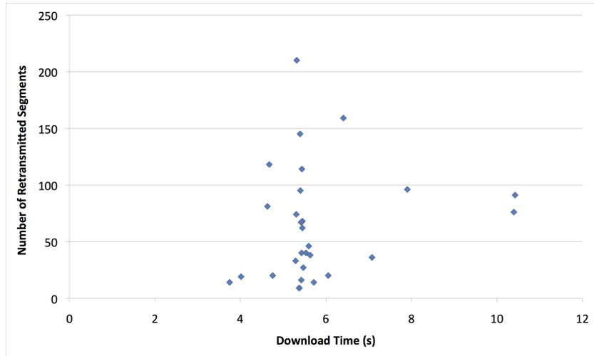
Figure 5.8: Impact of Retransmissions on Download Time (63 MB File, V/V)
