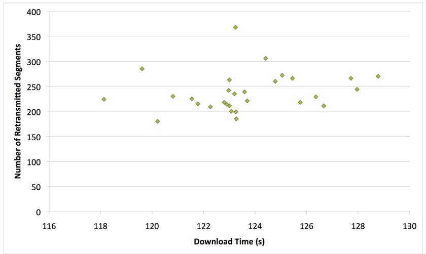
Figure 5.7: Impact of Retransmissions on Download Time (625 MB File, P/V)
