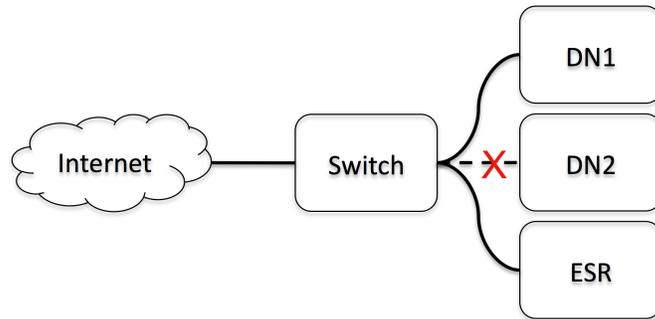
a) Failure of a single link, disconnecting a single DN
