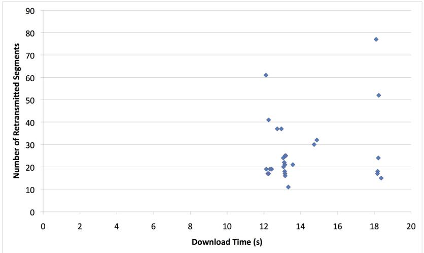
Figure 5.6: Impact of Retransmissions on Download Time (63 MB File, P/V)
