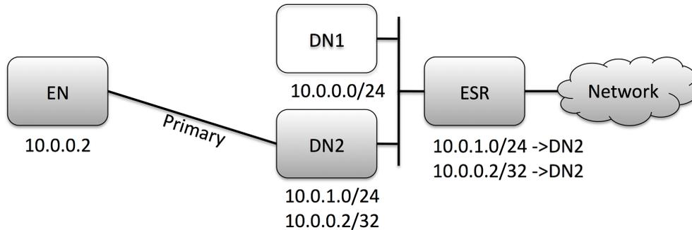
b) DN1 has failed, traffic redirected through DN2
