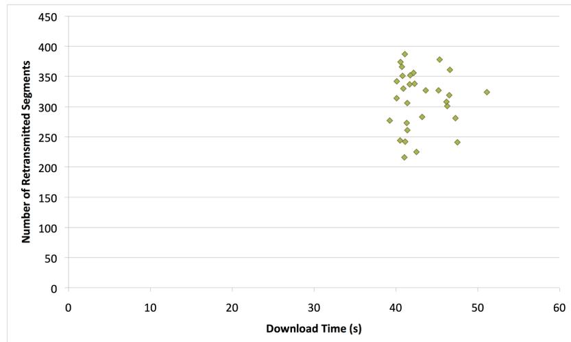
Figure 5.9: Impact of Retransmissions on Download Time (625 MB File, V/V)
