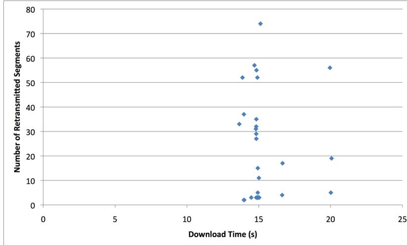
Figure 5.4: Impact of Retransmissions on Download Time (63 MB File, P/P)
