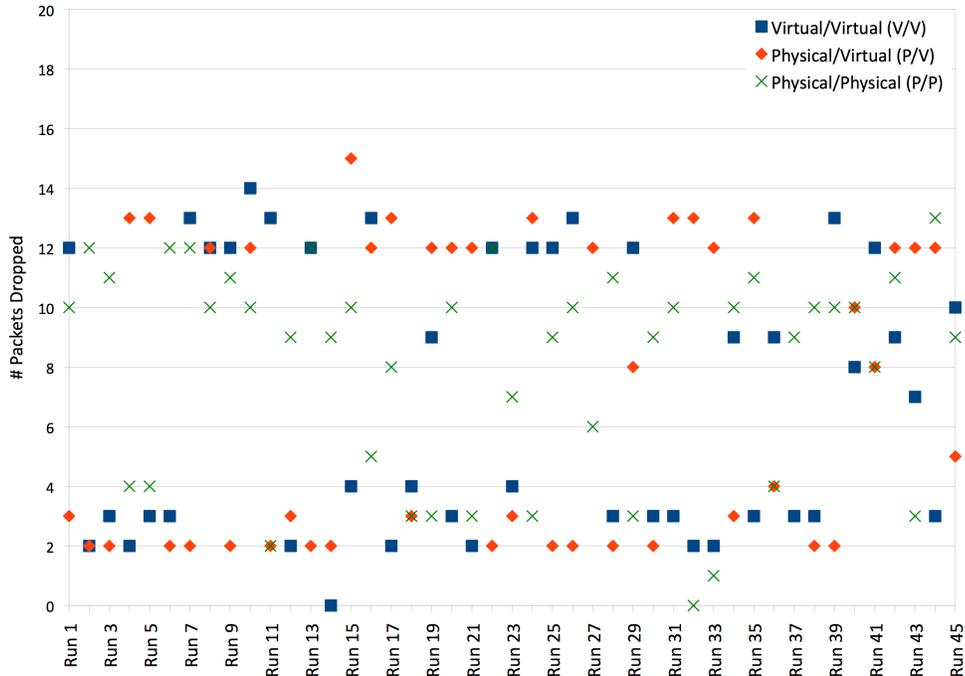
Figure 5.3: Packet Drop Count During A Failover (Rate of 10 Packets Per Second)
