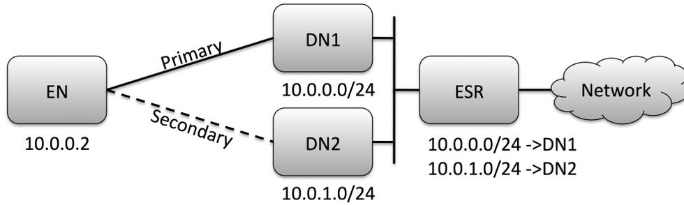
a) EN connected to both DNSs, traffic flowing through DN1
