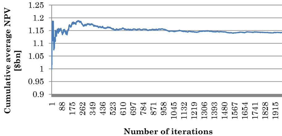
**Figure 5-12. Cumulative average NPV over 2000 iterations.**
