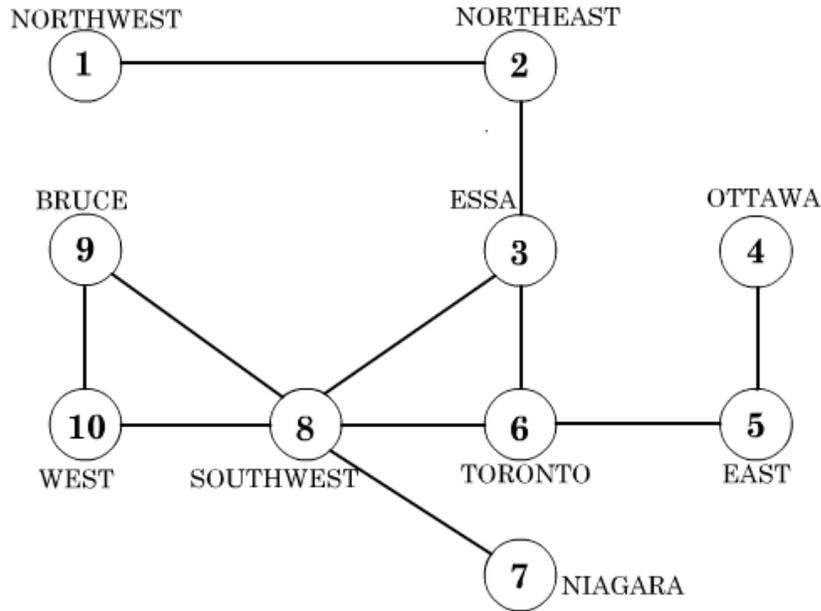
**Figure 4-5: Simplified transmission network model.**
