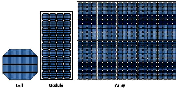
Figure 2-2. Depiction of PV system modularity.
