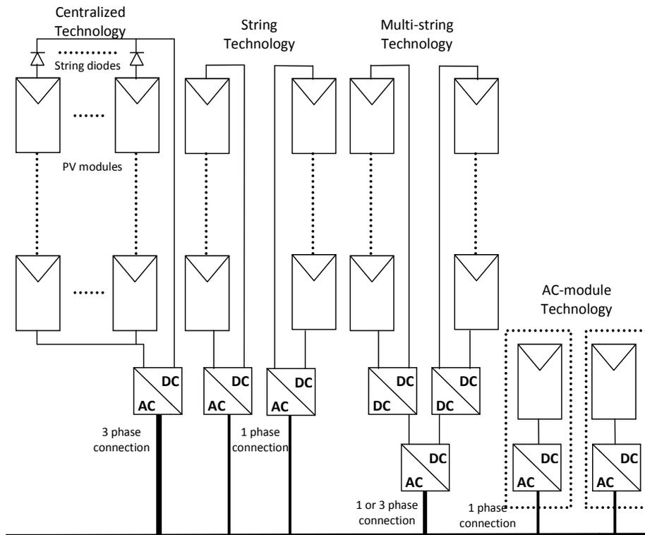
Figure 2-3. Historical overview of the PV system inverter topology [26].
