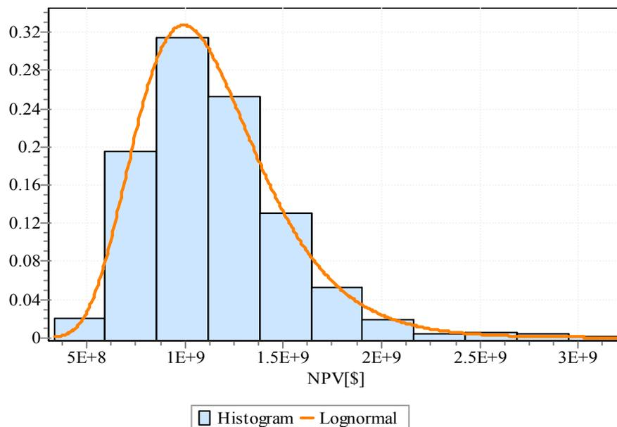
**Figure 5-13. Histogram and best-fit probability distribution function of NPV over 2000 iterations.**
