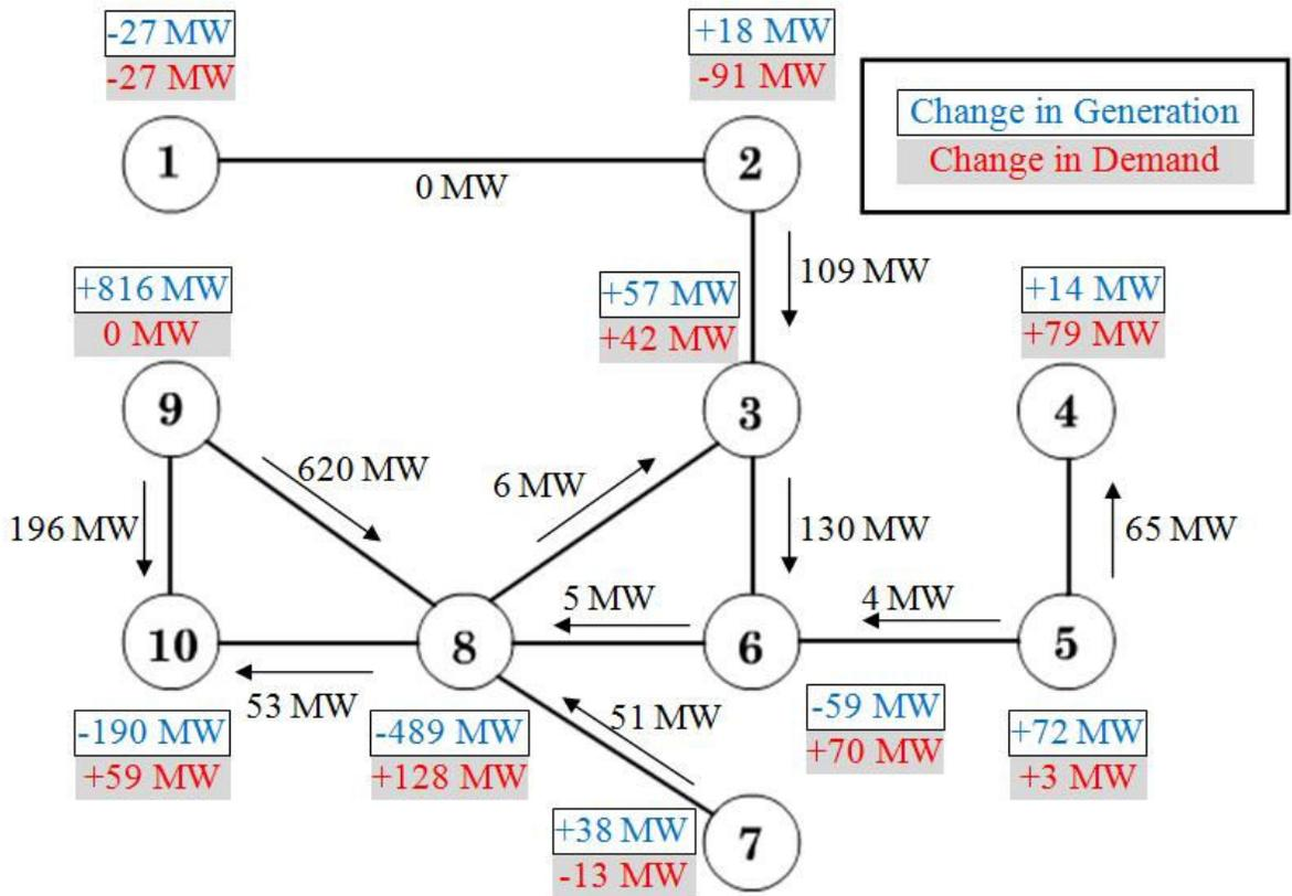
**Figure 5-2. Transmission line flows, generation and demand changes 2010-2018.**
