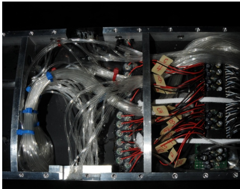
Figure 2.20: Detailed view of midspan instrumentation, including a cluster of static pressure taps, microphone array, and amplification bus.
