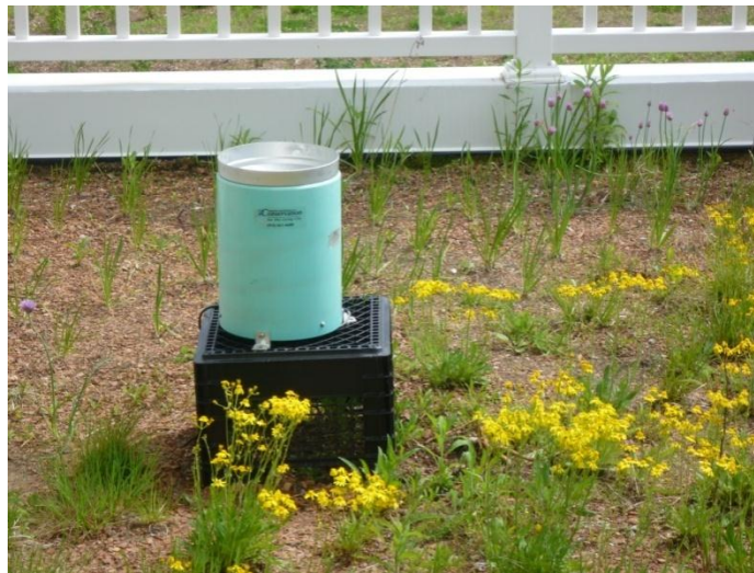
Figure 11: Tipping bucket rain gauge located on the greenroof.
