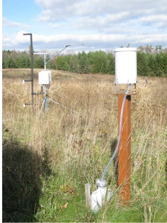
Figure 12: Meteorological station containing rain gauge located 450 m from greenroof.
