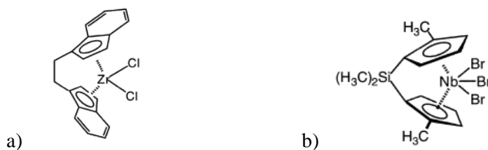
Figure 2.5 Typical metallocene catalysts, a) dichloro[1,2-di( \eta^5 -inden-1-yl)ethane]zirconium b) tribromo[2,2'-(dimethylsilanediy)l]-di( \eta^5 -cyclopentadienyl)niobium (Salzer, 1999).
