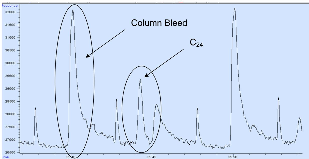
**Figure 3-3:** A fragment of a 2D gas chromatogram of an alkane mixture showing the n-C<sub>24</sub> peak (11 µg/L) with a temperature program of 3 °C/min and a modulation period of six seconds.
