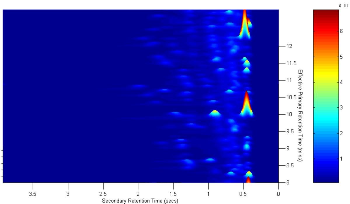
**Figure 5-14:** Three dimensional view of diesel fuel in CS<sub>2</sub> (10:1 dilution) for the CMt67 modulator
