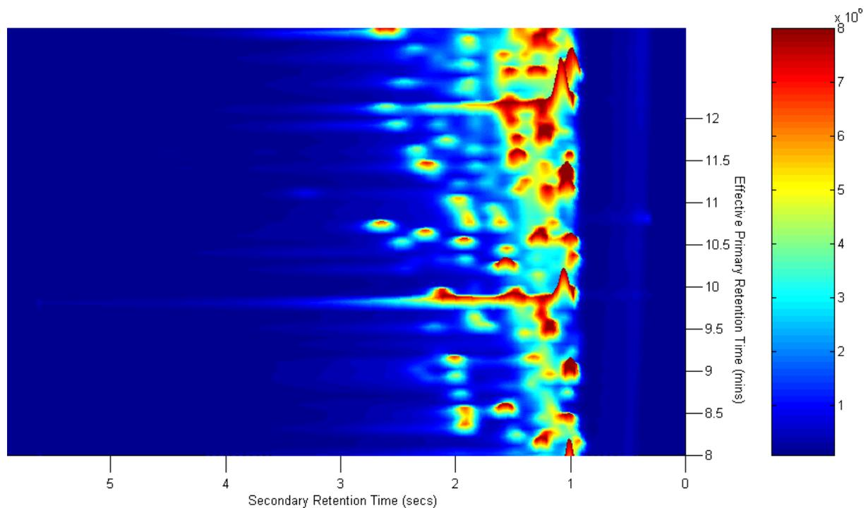
**Figure 5-15:** Three dimensional view of diesel fuel in CS<sub>2</sub> (10:1 dilution) for the CMS66 modulator
