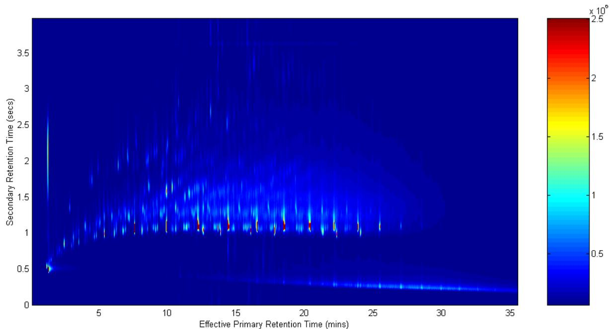
**Figure 5-7:** A two-dimensional chromatogram of a solution of diesel fuel in CS<sub>2</sub> (1:10 dilution) using CMt66
