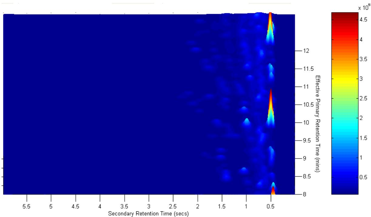
**Figure 5-12:** Three dimensional view of diesel fuel in CS<sub>2</sub> (10:1 dilution) for the CM67 modulator
