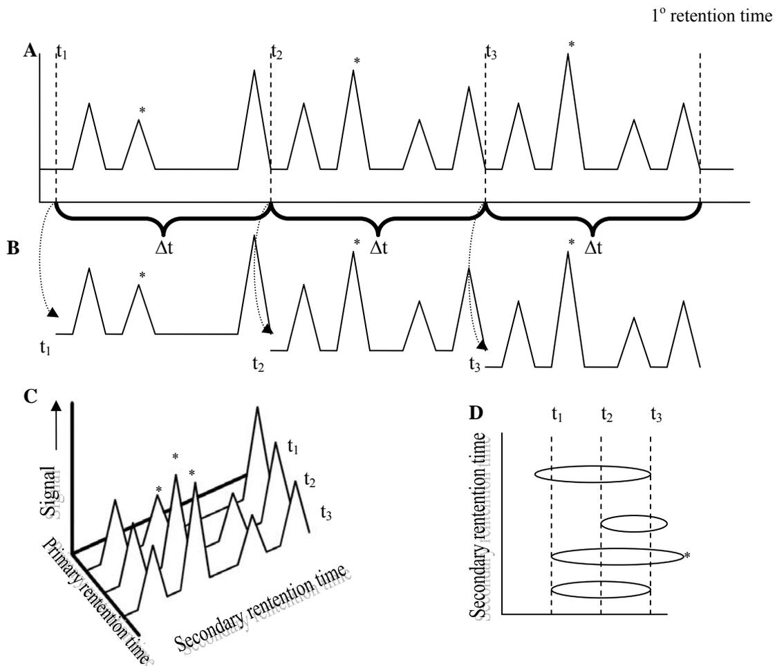
**Figure 1-4:** Data interpretation in GC  $\times$  GC. (A) The chromatogram is recorded by the detector along with the injection times ( $t_1$ ,  $t_2$ , and  $t_3$ ) into the secondary column. The modulation time is represented by  $\Delta t$ . (B) The chromatogram is cut into individual "slices" using computer software. (C) The individual second dimension chromatograms are then aligned to produce a 3-D chromatogram. (D) A top down view of the 3-D chromatogram (based on ref.<sup>10</sup>).
