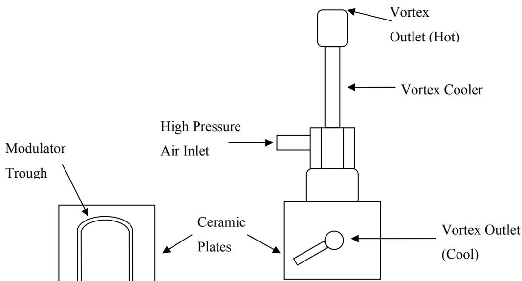
**Figure 2-1:** Block diagram of the modulator mount, used to secure and cool the modulator
