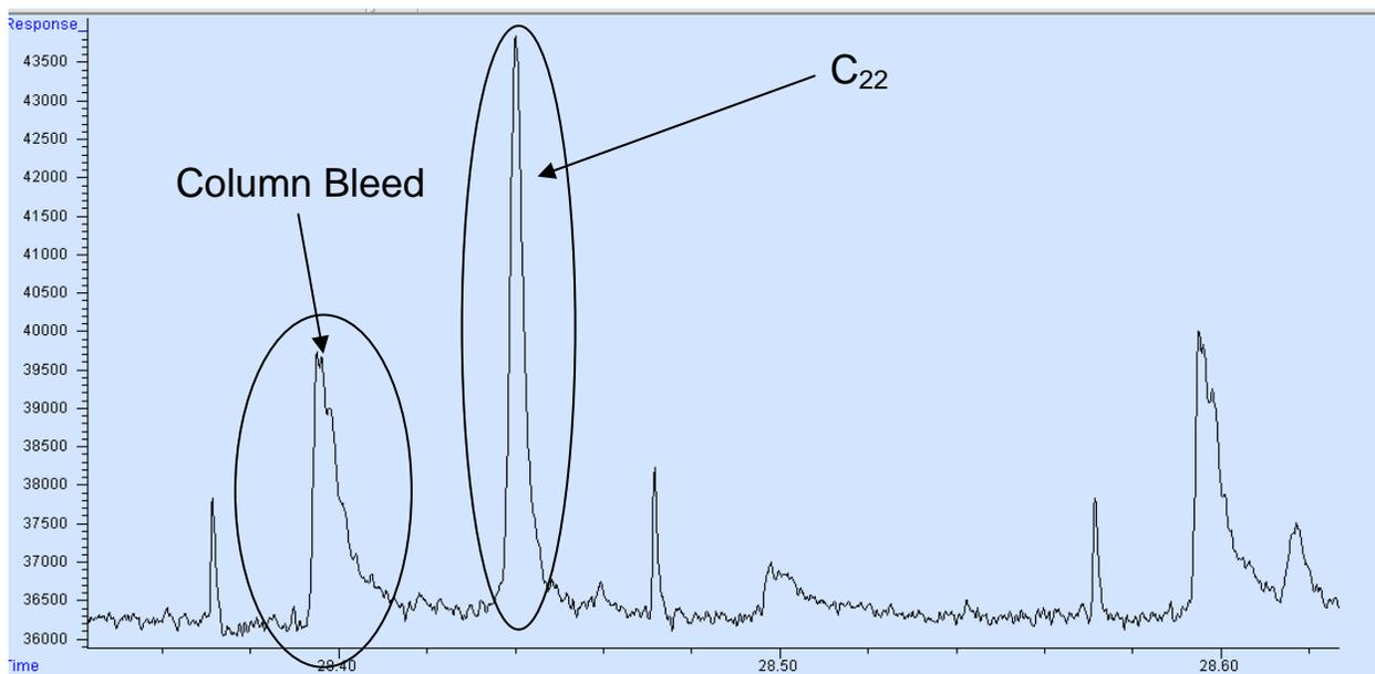
**Figure 3-4:** A fragment of a 2D gas chromatogram of an alkane mixture showing the n-C<sub>22</sub> peak (8.5 µg/L) with a temperature program of 3 °C/min and a modulation period of 12 seconds.
