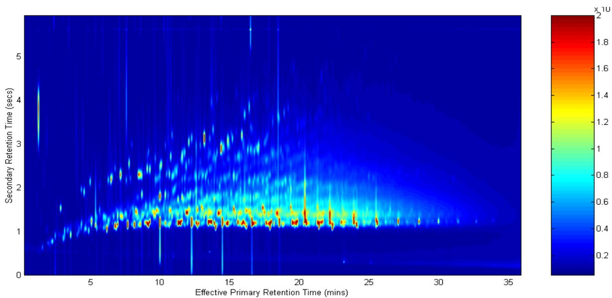
**Figure 5-5:** A two-dimensional chromatogram of a solution of diesel fuel in CS<sub>2</sub> (1:10 dilution) using CM66.
