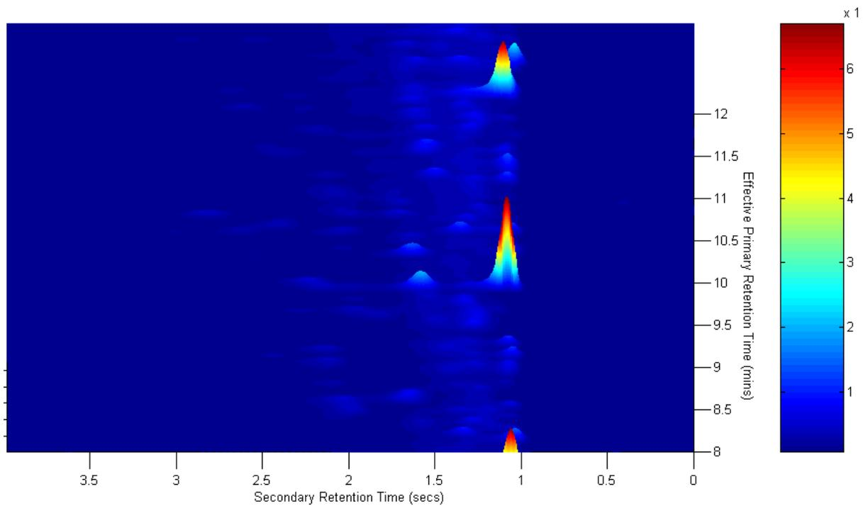
**Figure 5-13:** Three dimensional view of diesel fuel in CS<sub>2</sub> (10:1 dilution) for the CMt66 modulator
