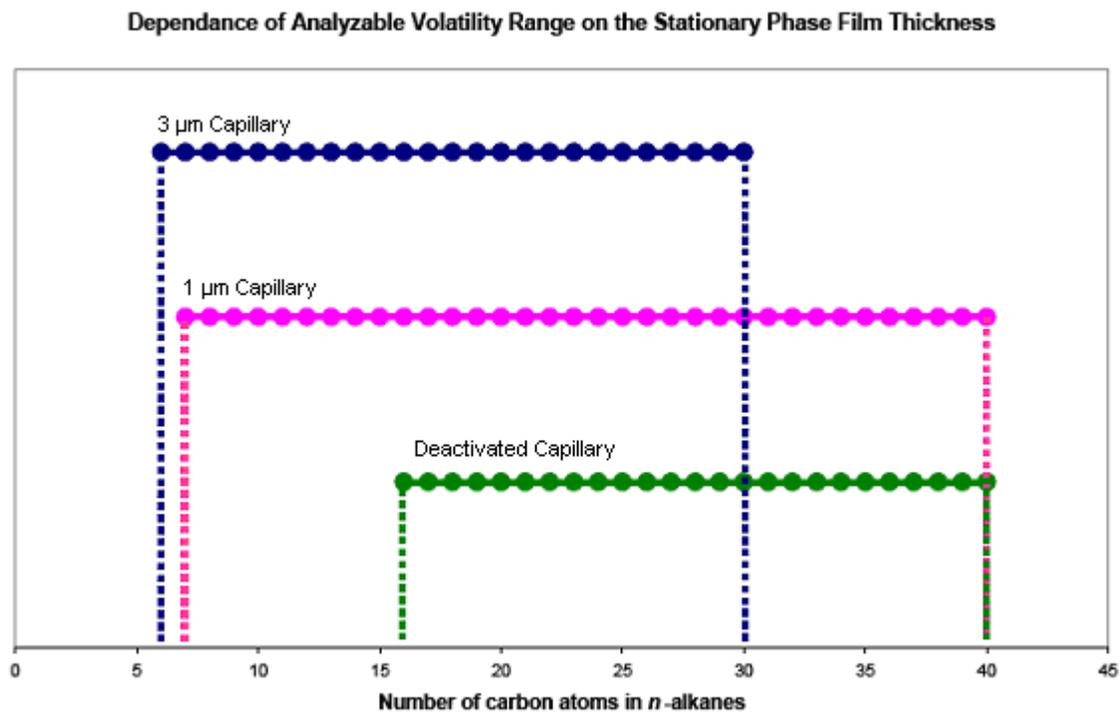
**Figure 1-9:** A diagram of the ranges of n-alkanes that could be effectively modulated with the traps coated with the stationary phases of different thicknesses.<sup>9</sup>
