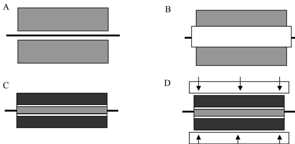
**Figure 2-2:** Block diagram of how to flatten capillaries in order to produce modulators. A capillary (black) is placed (A) between two shims (light grey) and then taped (white) in place (B). The apparatus from part B is then placed (C) between two parallels (dark grey), which are subsequently placed in a vice (D) where the capillary can be pressed until flattened to the proper thickness.
