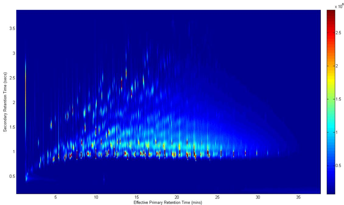
**Figure 5-8:** A two-dimensional chromatogram of a solution of diesel fuel in CS<sub>2</sub> (1:10 dilution) using CMt67
