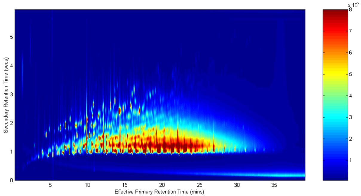
**Figure 5-9:** A two-dimensional chromatogram of a solution of diesel fuel in CS<sub>2</sub> (1:10 dilution) using CMS66
