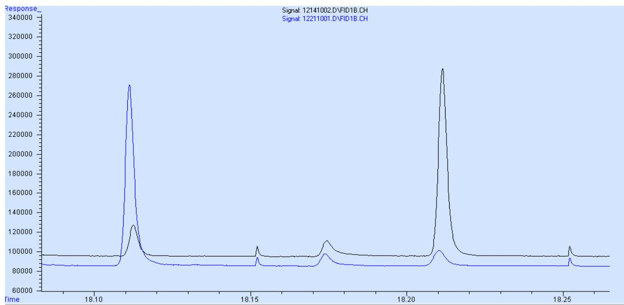
**Figure 6-2:** Chromatogram of  $C_{20}$ , at the beginning of the robustness test in black (right) and end of the test in blue (left)
