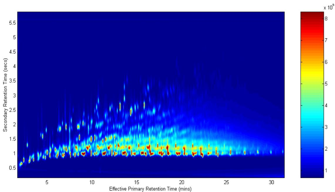
**Figure 5-6:** A two-dimensional chromatogram of a solution of diesel fuel in CS<sub>2</sub> (1:10 dilution) using CM67
