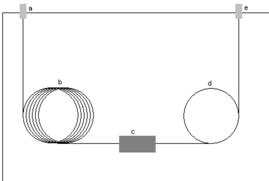
**Figure 1-1** A block diagram of GC  $\times$  GC system; a) Injector; b) Primary Column c) Modulator; d) Secondary Column e) Detector <sup>10</sup>
