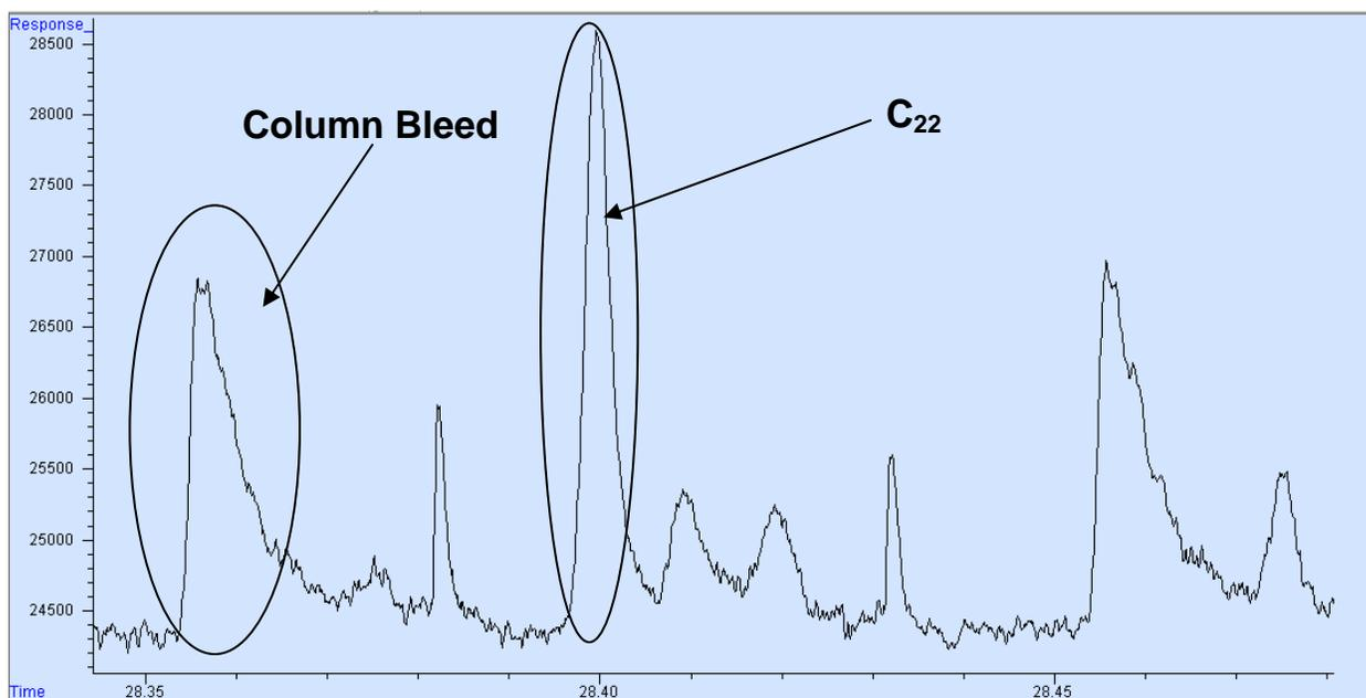
**Figure 3-2:** A fragment of a 2D gas chromatogram of an alkane mixture showing the n-C<sub>22</sub> peak (8.5 µg/L) with a temperature program of 3 °C/min and a modulation period of six seconds.
