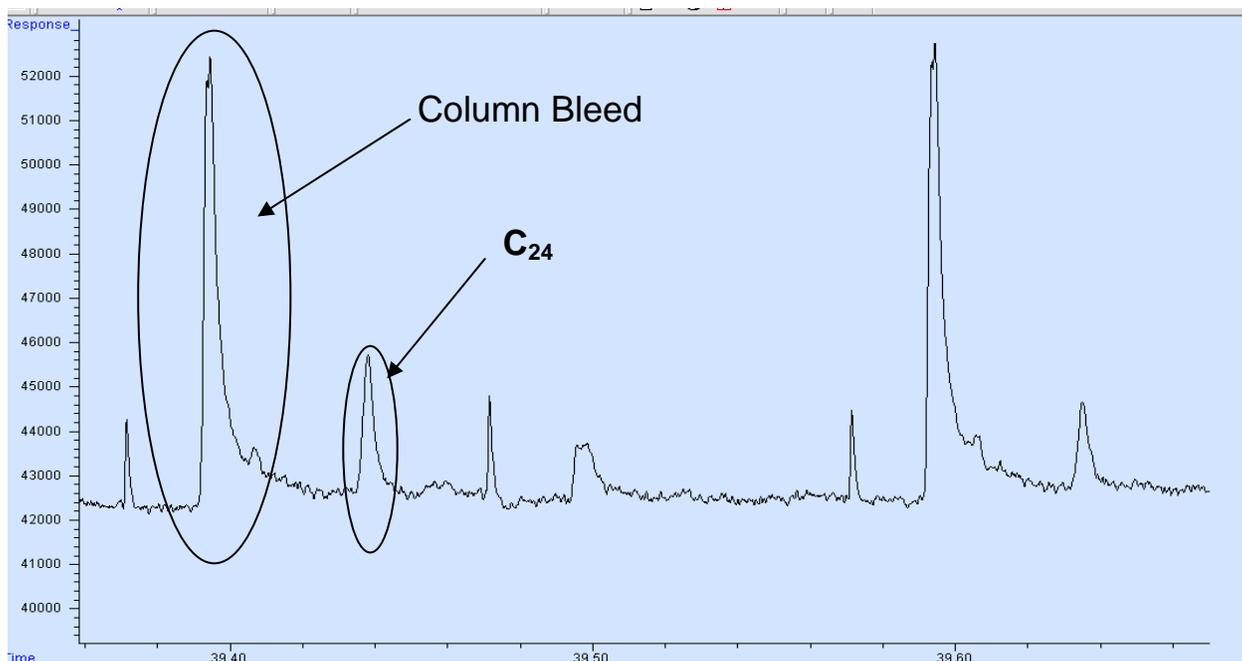
**Figure 3-5:** A fragment of a 2D gas chromatogram of an alkane mixture showing the n-C<sub>24</sub> peak (11 µg/L) with a temperature program of 3 °C/min and a modulation period of 12 seconds.
