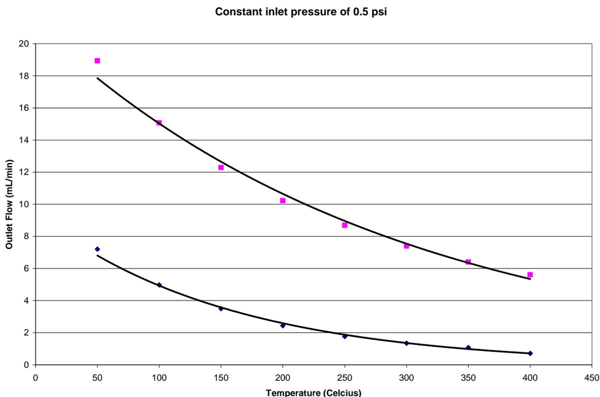
**Figure 5-3:** Experimental results for carrier gas flow rate through the modulator as temperature increased at a constant inlet pressure of 0.5 psi. A: results for the restricted modulator; B: theoretical results for an unrestricted modulator.
