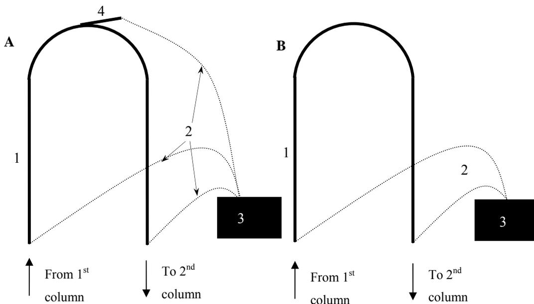
**Figure 5-1:** Schematic diagrams of the modulators. A: dual stage; B: single stage. 1) modulator tubing; 2) electrical leads; 3) power supply; 4) middle contact.
