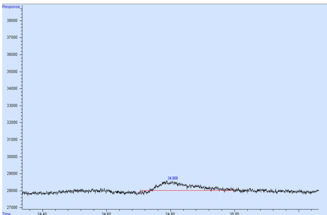
**Figure 3-1:** A fragment of a 1D gas chromatogram of an alkane mixture showing the n-C<sub>24</sub> peak (150 ug/L) with a temperature program of 3 °C/min.
