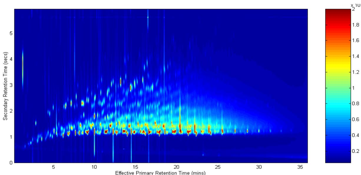
**Figure 5-4:** A two-dimensional chromatogram of a solution of diesel fuel in CS<sub>2</sub> (1:10 dilution) using CM66.
