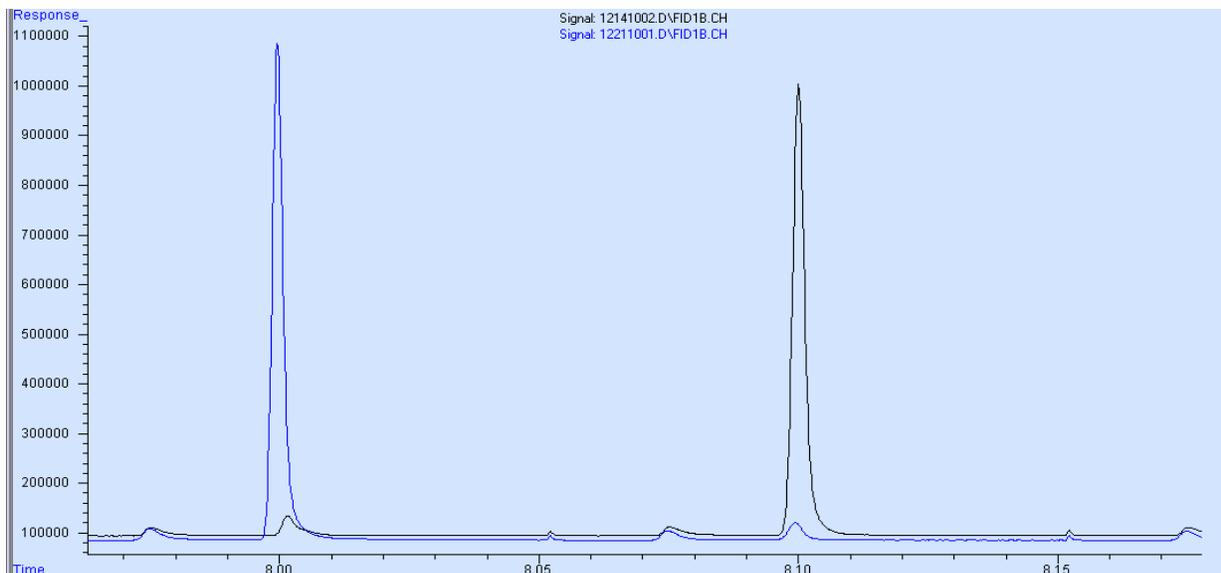
**Figure 6-1:** Chromatogram of  $C_{16}$  at the beginning of the robustness test in black (right) and end of the test in blue (left)
