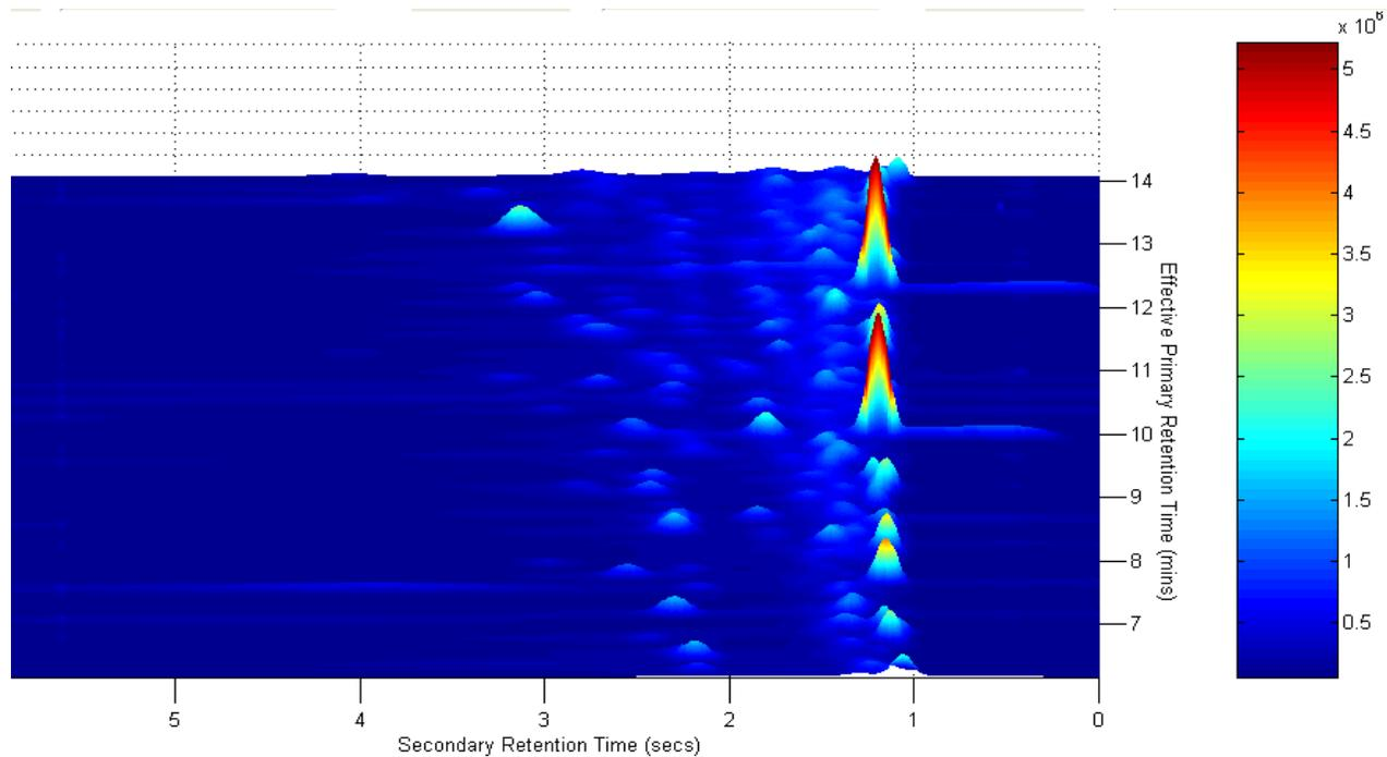
**Figure 5-11:** Three dimensional view of diesel fuel in CS<sub>2</sub> (10:1 dilution) for the CM66 modulator
