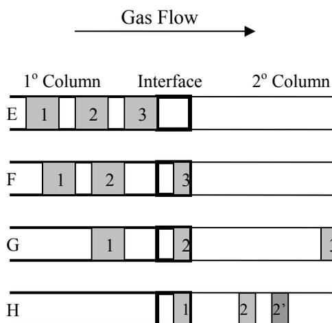
**Figure 1-3:** A diagram of two columns with a modulator<sup>10</sup>
