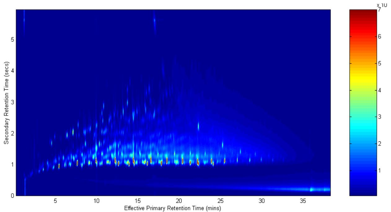
**Figure 5-10:** A two-dimensional chromatogram of a solution of diesel fuel in CS<sub>2</sub> (1:10 dilution) using CMS67
