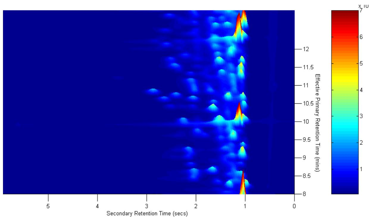
**Figure 5-16:** Three dimensional view of diesel fuel in CS<sub>2</sub> (10:1 dilution) for the CMS67 modulator
