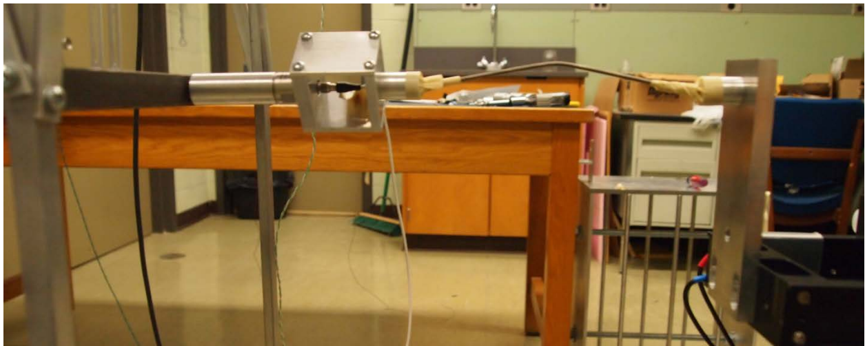
Figure E. 13: Stinger assembly after excessive load
