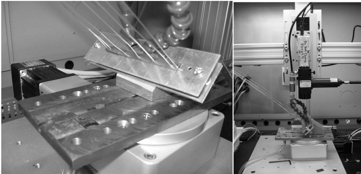
Figure 3-7: Pulsed Nd:YAG laser welding system used to spot weld the thermocouples to the steel spacer.
