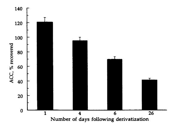
to drop. At 6 days the amount of ACC recovered was 69.9%, athough the high standard error suggests that this number may be low, and by 26 days the ACC content had dropped to 41.6% of the amount measured immediately following derivatization and the chromatogram of the sample also showed several new peaks suggesting breakdown of ACC. In the remainder of this study, all samples were analyzed within one day of being derivatized.
