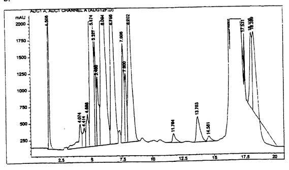
reconditioned for the next sample during the last 12 minutes of the Water's gradient, which had a total run time of 45 minutes. Modification of the Water's gradient resulted in a reduction in the total run time from 45 to 23 minutes and improved separation of the ACC peak from the surrounding peaks.
