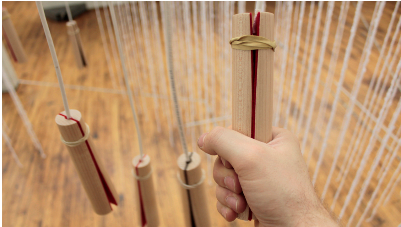
fig. 8.10 Force-sensing handles. Hand-crafted & finished maple with felt linings.
