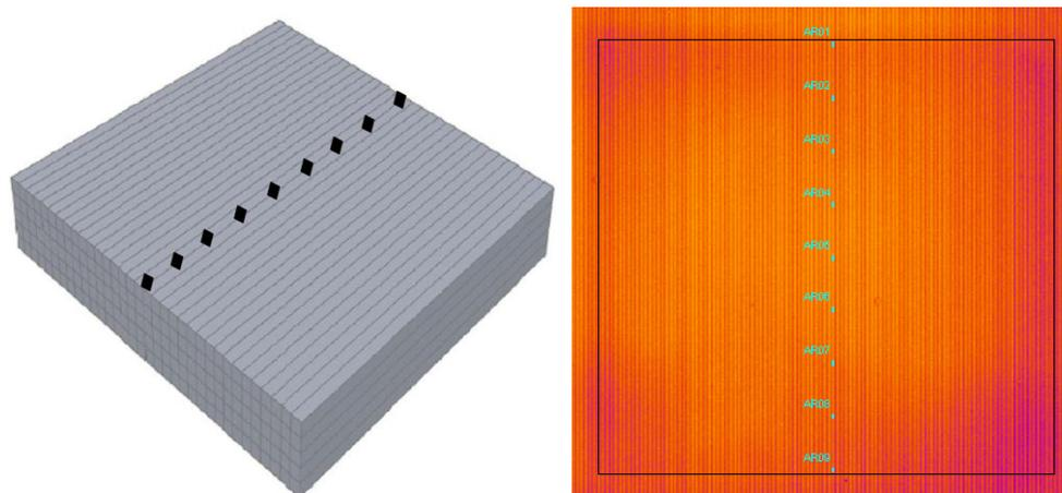
Figure 3. Schematic of data point distribution and an IR camera image (catalyst outlined in black)<sup>130</sup>.
