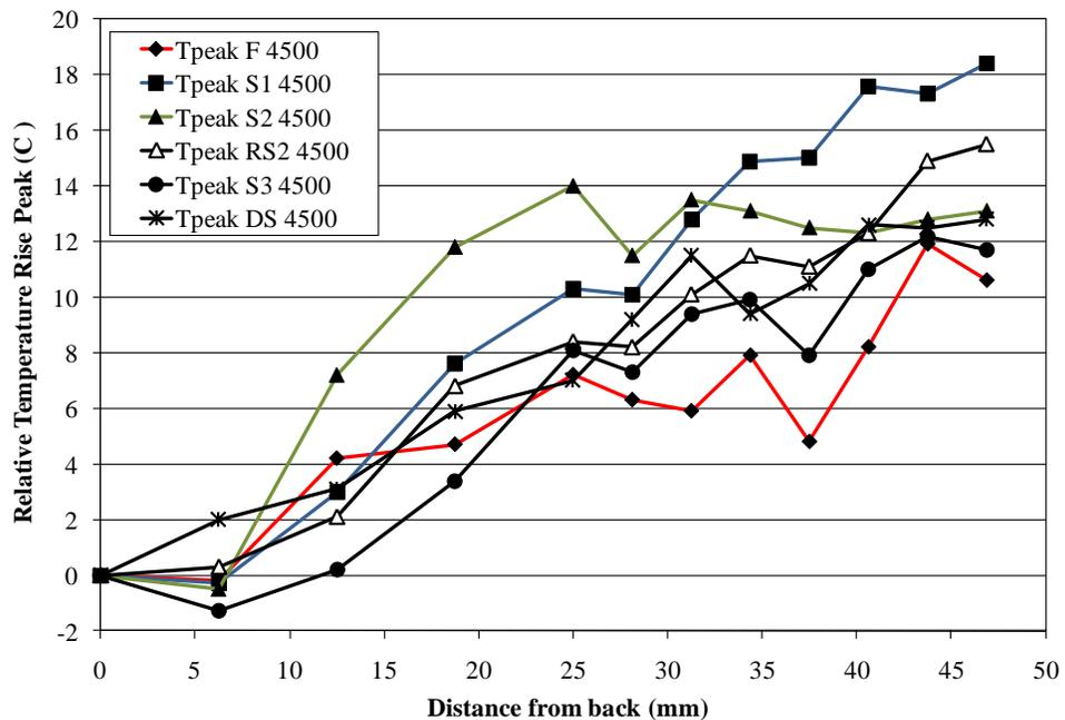
Figure 17. Relative temperature rise peak values as a function of position from the catalyst outlet, with the gas composed of 4500 ppm propylene, 6.5% O<sub>2</sub>, 4% H<sub>2</sub>O, 300 ppm He, and a balance of N<sub>2</sub>.
