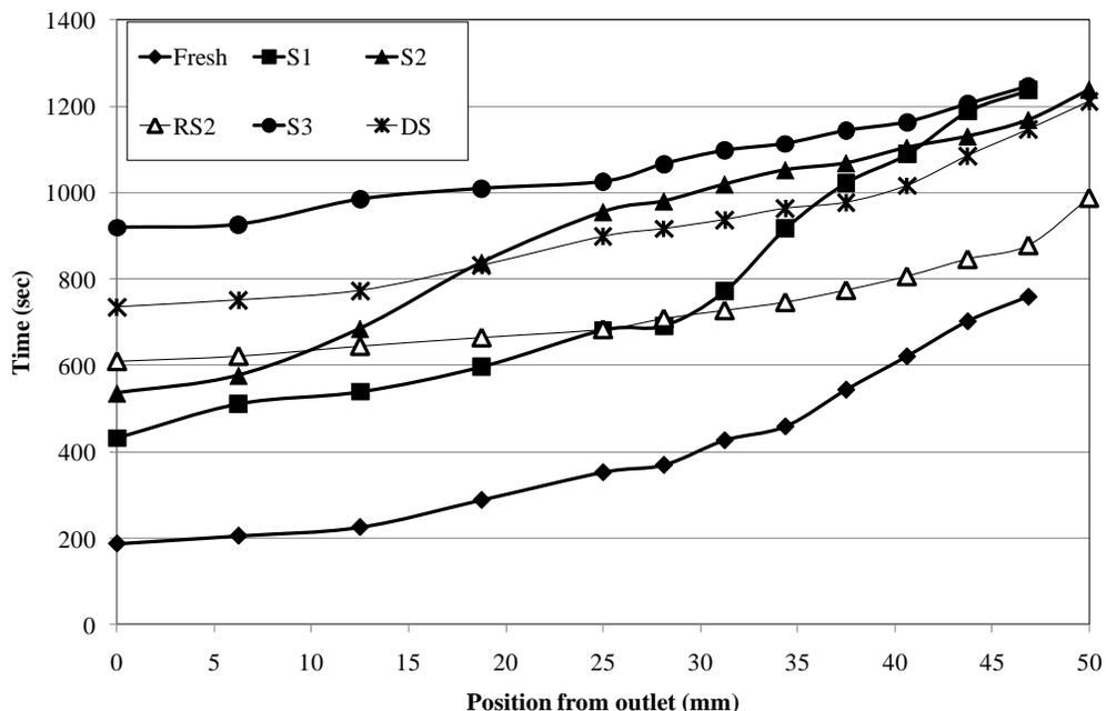
Figure 16. Time between the reference temperature and the temperature peak measured at different catalyst positions. The reactor feed consisted of 1500 ppm propylene, 6.5% O<sub>2</sub>, 4% H<sub>2</sub>O, 300 ppm He, and a balance of N<sub>2</sub>.
