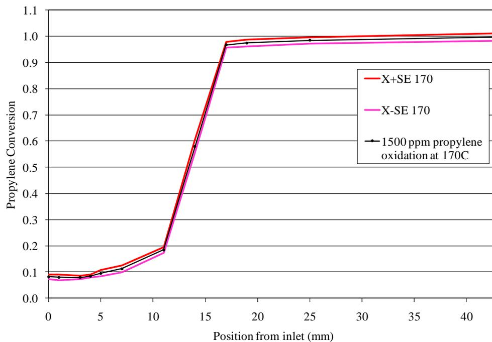
Figure 22. Calculated confidence interval on reaction zone at 170°C. The gas composition was 1500 ppm propylene, 6.5% O<sub>2</sub>, 4% H<sub>2</sub>O, 300 ppm He, and a balance of N<sub>2</sub>.
