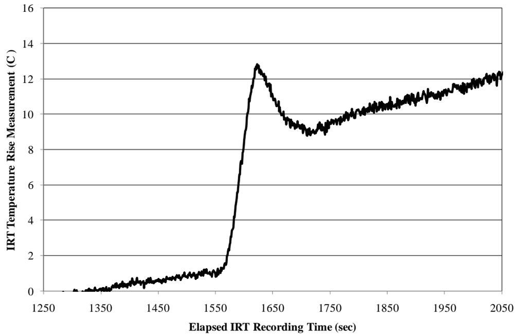
Figure 5. Sample TPO temperature rise profile following subtraction of the inert feed temperature ramp.
