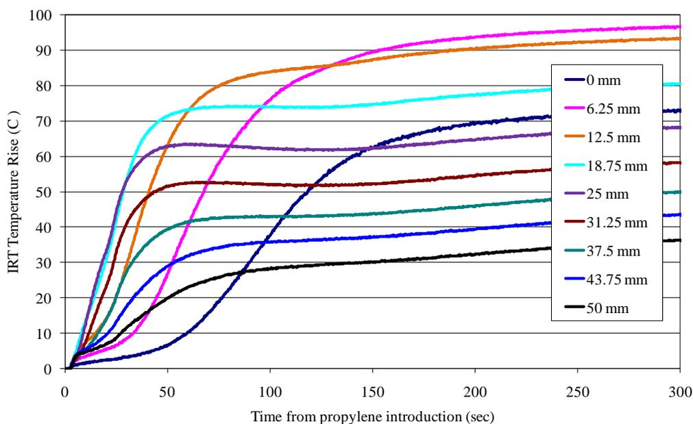
Figure 12. IRT Temperature rise light-off sample. From 207°C steady-state with 4500 ppm propylene, 6.5% O<sub>2</sub> and balance N<sub>2</sub> with the catalyst condition A1.
