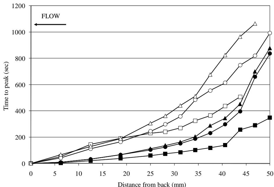
Figure 9. Time between the temperature peak measured at the most downstream position and the temperature peak at different upstream positions, during TPO with 4500 ppm (closed points) and 1500 ppm (open points) propylene. Catalyst F designated by square points (□), A1 by circle points (O), and A2 by triangle points (Δ).
