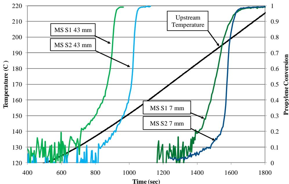
Figure 14. Combined propylene conversion profiles during TPO. Data were obtained from the S1 and S2 catalysts, and the gas composition contained 1500 ppm propylene, 6.5% O<sub>2</sub>, 4% H<sub>2</sub>O, 300 ppm He, and a balance of N<sub>2</sub>.
