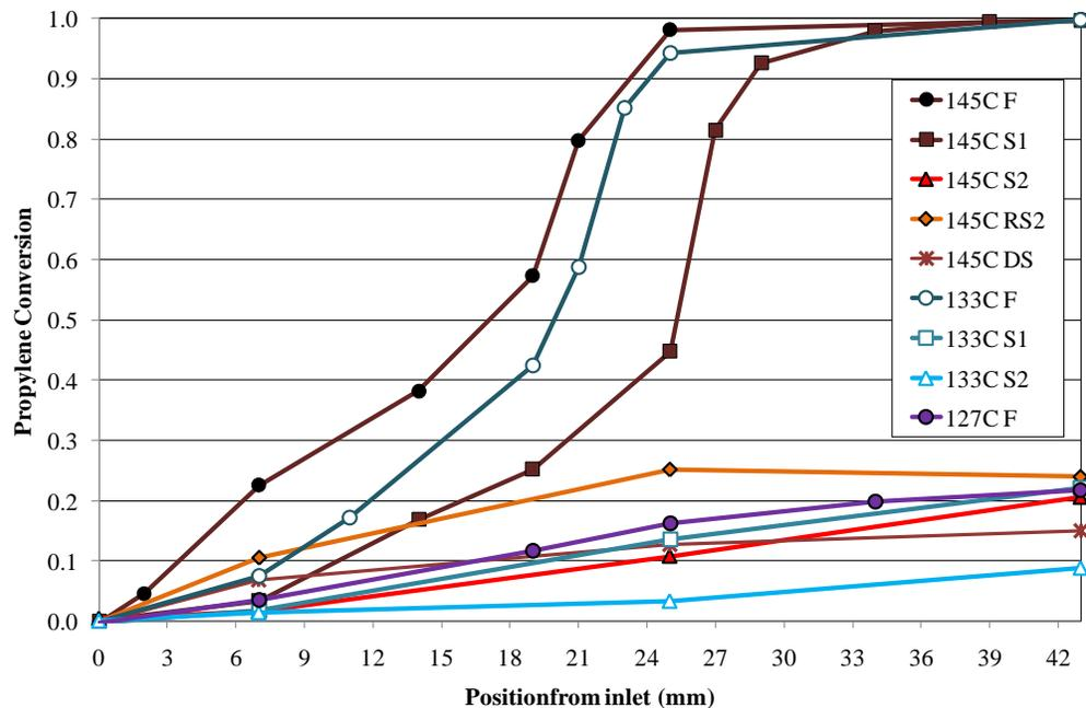
Figure 20. Low temperature steady-state, spatially-resolved conversion profiles over the first 43 mm of catalyst (last point measured). The gas composition was 1500 ppm propylene, 6.5% O<sub>2</sub>, 4% H<sub>2</sub>O, 300 ppm He, and a balance of N<sub>2</sub>.
