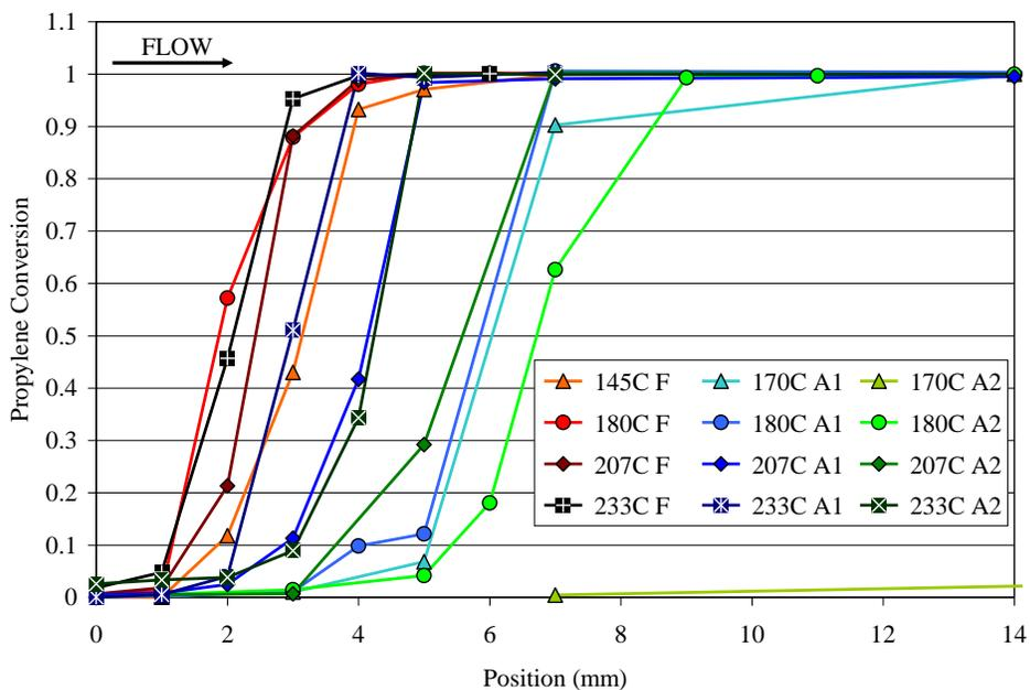
Figure 11. Steady-state, spatially-resolved conversion profiles over the first 14 mm of catalyst. The gas composition was 4500 ppm propylene, 6.5% O<sub>2</sub>, 4% H<sub>2</sub>O, 300 ppm He, and a balance of N<sub>2</sub>. Note that the x-axis is now relative to the upstream face (0 mm is the catalyst inlet).
