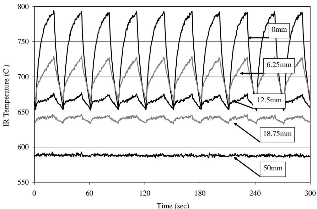
Figure 6. Example temperature data set obtained during heterogeneous aging (A1).
