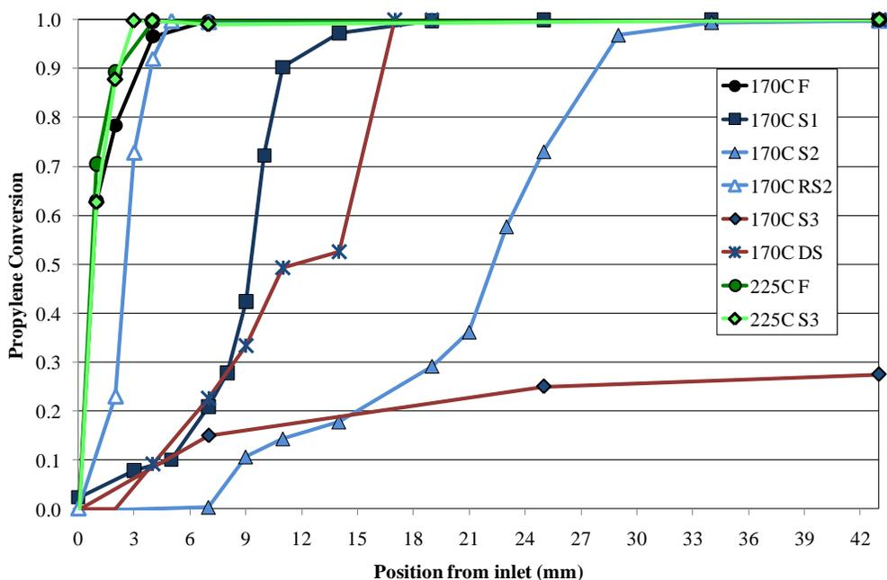
Figure 21. Steady-state, spatially-resolved conversion profiles over the first 43 mm of catalyst (last point measured). The gas composition was 1500 ppm propylene, 6.5% O<sub>2</sub>, 4% H<sub>2</sub>O, 300 ppm He, and a balance of N<sub>2</sub>.
