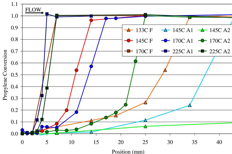
Figure 13. Steady-state, spatially-resolved conversion profiles over the first 43 mm of catalyst (last point measured). The gas composition was 1500 ppm propylene, 10% O<sub>2</sub>, 4% H<sub>2</sub>O, 300 ppm He, and a balance of N<sub>2</sub>.
