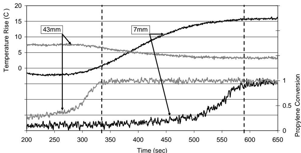
Figure 8. Combined temperature rise and propylene conversion data. Data were obtained from unaged catalyst, and the gas composition was 1500 ppm propylene, 6.5% O<sub>2</sub>, 4% H<sub>2</sub>O, 300 ppm He, and a balance of N<sub>2</sub>.
