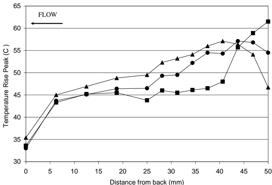
Figure 10. Temperature rise peak values as a function of position from the catalyst outlet, with the gas composed of 4500 ppm propylene, 6.5% O<sub>2</sub>, 4% H<sub>2</sub>O, 300 ppm He, and a balance of N<sub>2</sub>. Catalyst F designated by square points (□), A1 by circle points (○), and A2 by triangle points (Δ).
