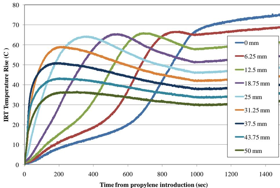
Figure 18. IRT temperature rise light-off sample. Inlet temperature was 180°C with 4500 ppm propylene, 6.5% O<sub>2</sub> and balance N<sub>2</sub> as the inlet gas composition, and the catalyst condition S2.
