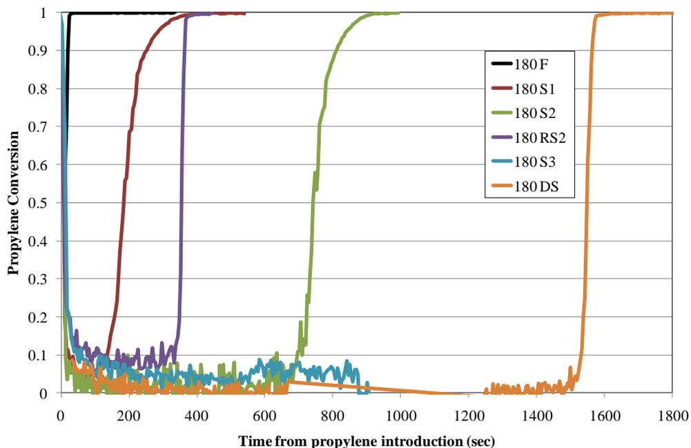
Figure 19. Time for conversion to reach 7 mm from the inlet during steady-state oxidation at 180°C. The gas was composed of 4500 ppm propylene, 6.5% O<sub>2</sub>, 4% H<sub>2</sub>O, 300 ppm He, and a balance of N<sub>2</sub>.
