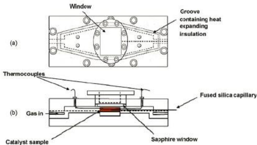
Figure 1. Schematic of the reactor; (a) top view and (b) side view<sup>75</sup>.
