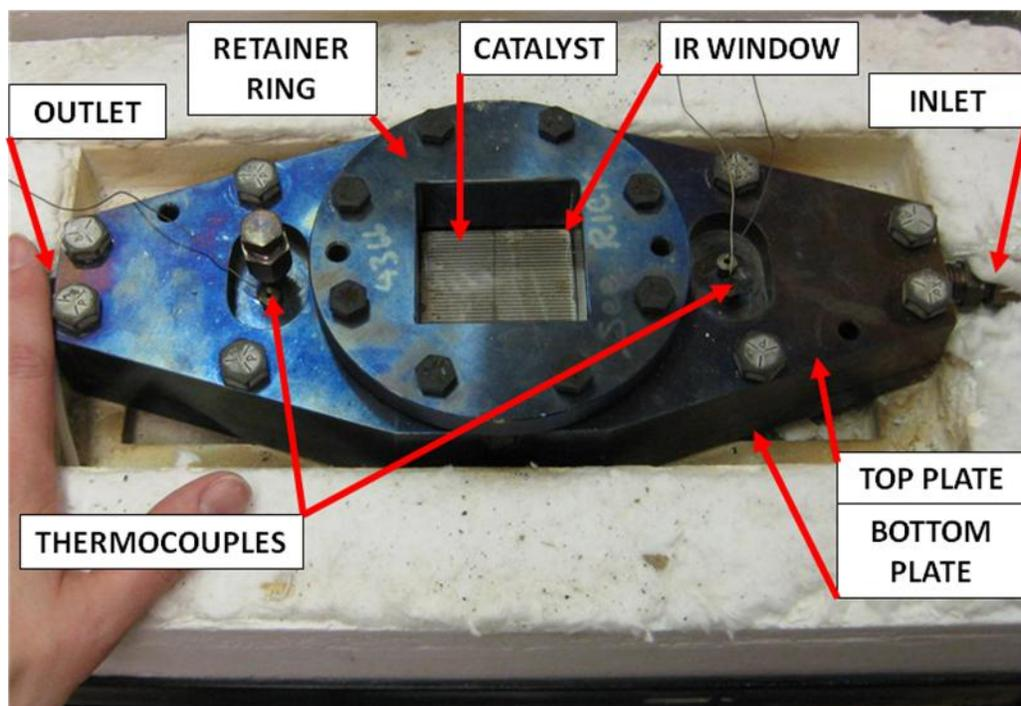
Figure 2. Top view of the IRT custom reactor.
