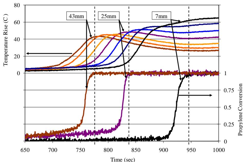
Figure 7. Combined temperature rise and propylene conversion data. Data were obtained from the unaged catalyst, and the gas composition was 4500 ppm propylene, 6.5% O<sub>2</sub>, 4% H<sub>2</sub>O, 300 ppm He, and a balance of N<sub>2</sub>.
