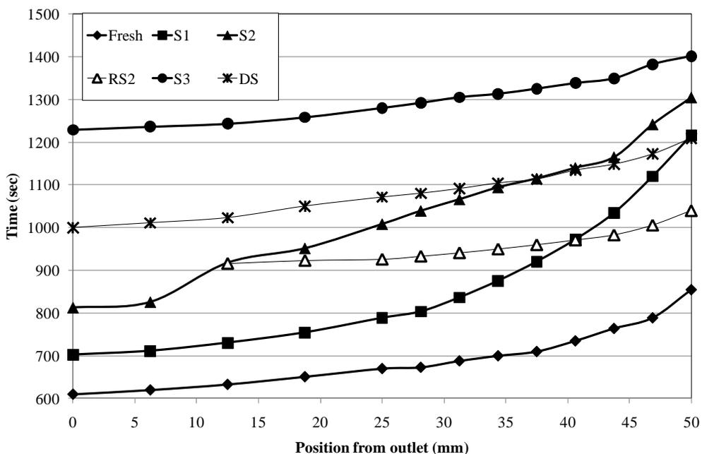
Figure 15. Time between the reference temperature and the temperature peak measured at different catalyst positions. The reactor feed consisted of 4500 ppm propylene, 6.5% O<sub>2</sub>, 4% H<sub>2</sub>O, 300 ppm He, and a balance of N<sub>2</sub>.
