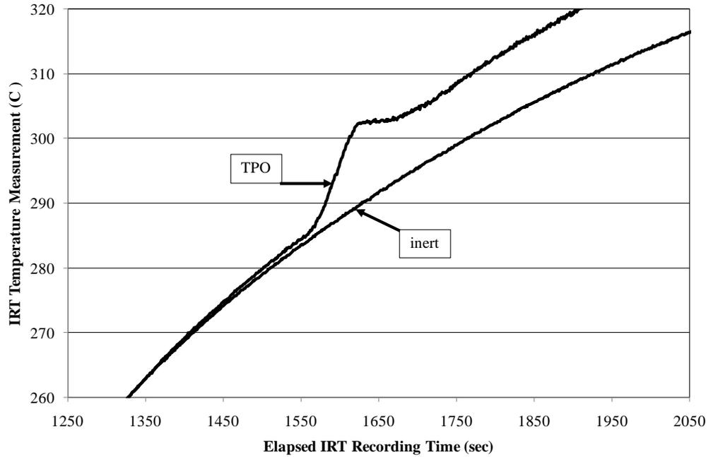
Figure 4. Sample TPO catalyst temperature data sets with and without propylene in the gas stream.
