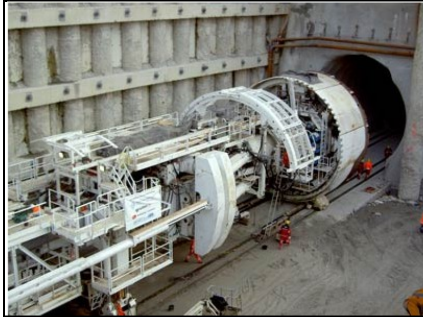
Fig.2.1 Tunnel boring machine (TBM) used to excavate cylindrical opening [AlpTransit Gotthard Ltd. http://www.alptransit.ch/pages/e/ ].
