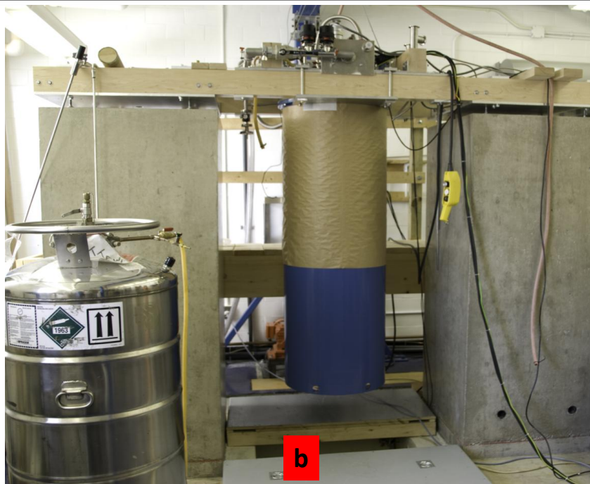
Figure 3.5: a) Schematic picture of the main parts of the Oxford dilution refrigerator. b) Real picture of the entire Oxford cryomagnetic system installation.
