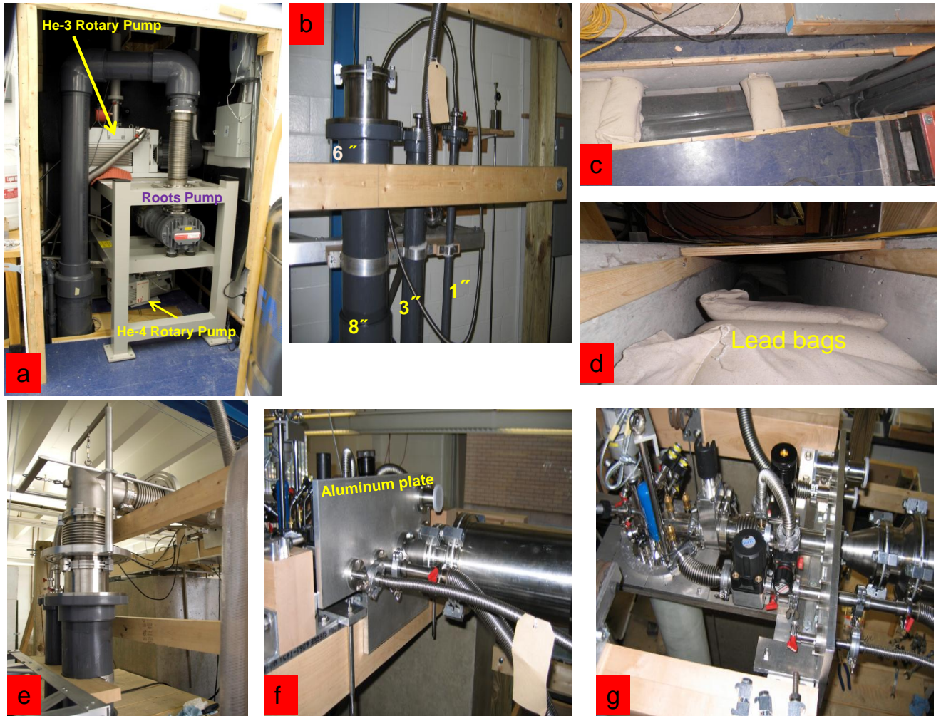
Figure 3.14: a) The pumps used in dilution fridge, they are acoustically isolated in a special room. b) Three different PVC pipes sizes have been used to connect the pumps to the fridge. c) and d) shows the trench in the ground used to contain the large size PVC pipes with lead bags to dump any introduced vibration. e) Double gimbal design. f) and g) shows the plate used to connect the Pumps to the dilution unit insert.
