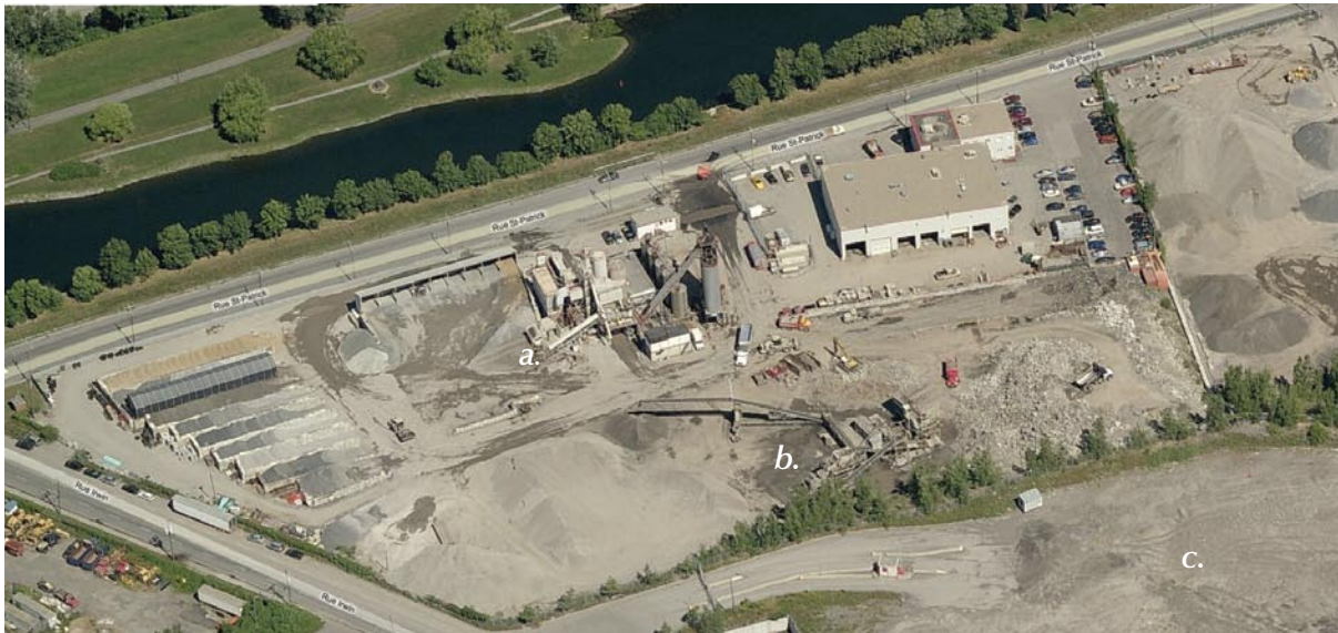
fig. 2.09, below: Bird's eye view of: a) asphalt paving production plant, b) aggregate recycling operations, and c) snow dump site atop a former coal gasification site at the Lachine-Turcot District. Image courtesy Bing Maps, 2009.
