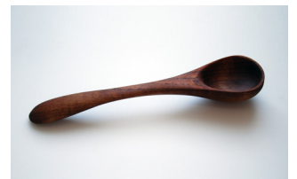
Fig 4.10 From block to spoon. Step 1 (top) - block of wood with outline of spoon drawn in pencil Step 2 - Cut outline using bandsaw Step 3 - Smooth spoon blank with belt sander Step 4 - Spoon finished using knife and sandpaper
