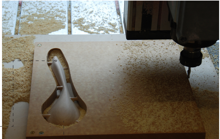
6) Carve using CNC Milling Machine
