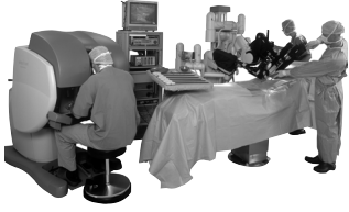
Fig 5.4 da vinci Standard Surgical System The operating surgeon sits at left.
