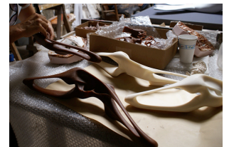
Fig 1.6 SLA originals (right) and wax duplicates.
