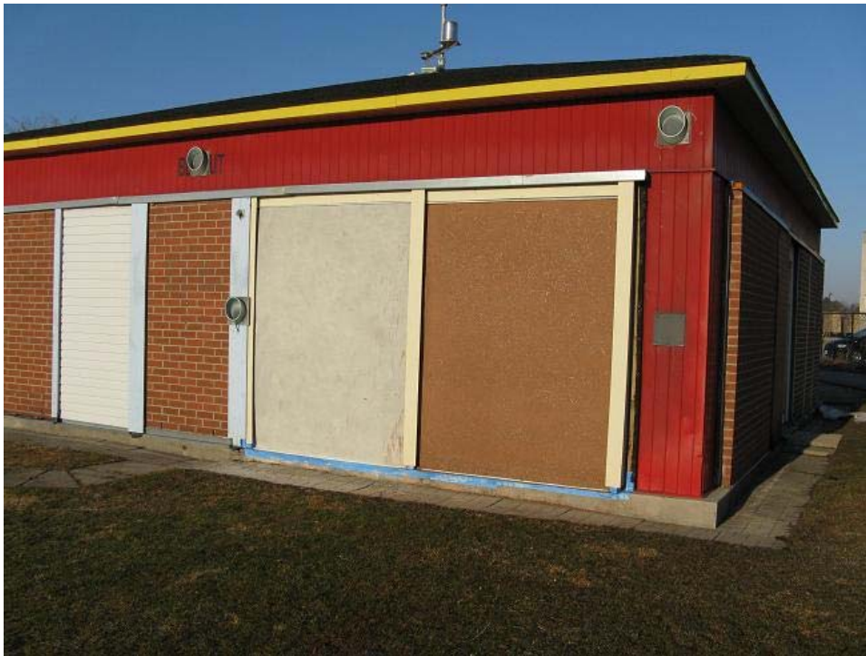
Figure 43. Finished test walls.
