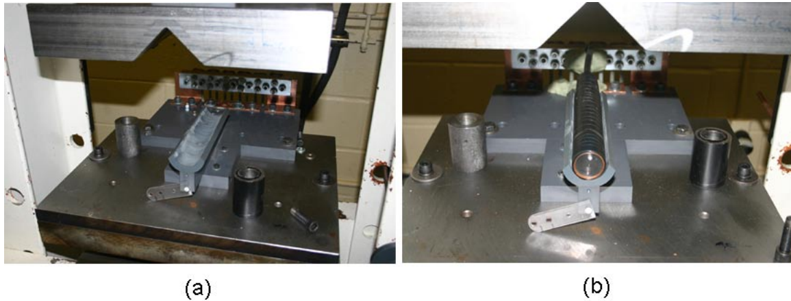
Figure 58: Photographs showing a) the PVC base of the connector and b) shows the base with the coil in place.
