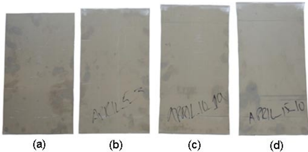
Figure 41: Images showing a) 203 x 356 mm (8 x 14") sheet cut from as-received material prior to stretching, and stretched to b) 5%, c) 10 %, and d) 15 %.
