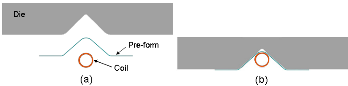
Figure 34: Schematic of the EM corner fill step of the hybrid process.
