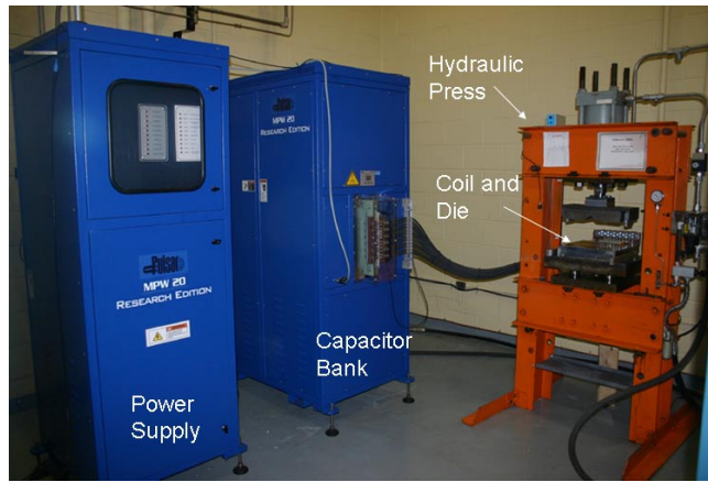
Figure 36: Experimental apparatus showing the MPG and hydraulic press used.
