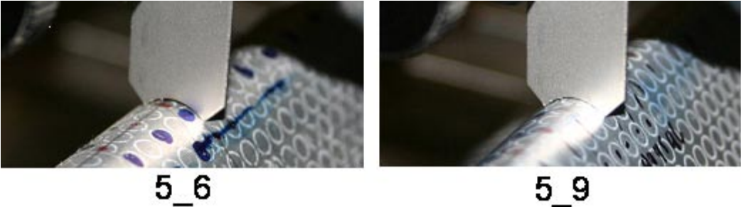
Figure 106: Close up of the centre region of the samples formed from the 5% pre-strained sheet with a 5 mm radius gauge.
