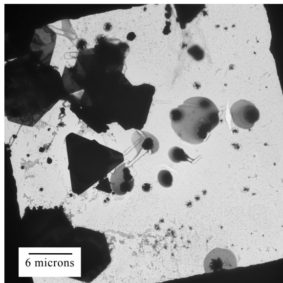
Figure 4.9: A TEM image of gold microplates.
