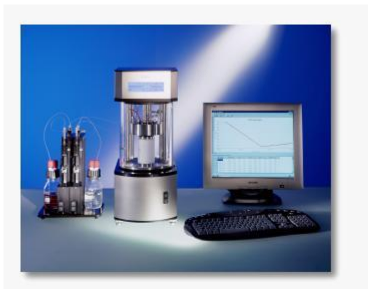
Figure 3.2 DCAT equipment for surface tension measurements [123]
