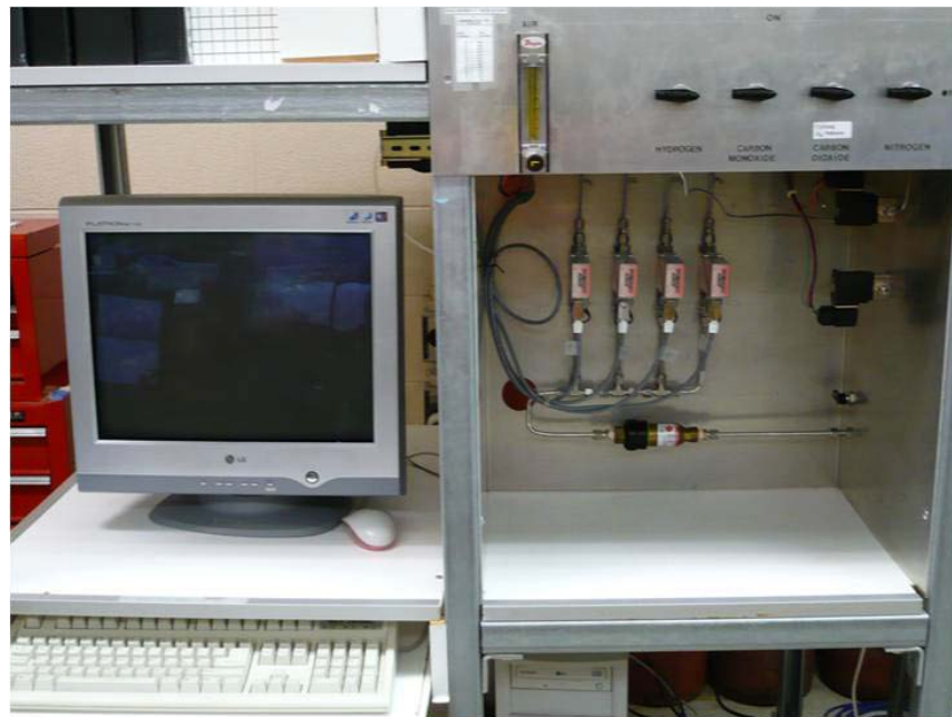
Figure 3-8 Flow controllers placed next to the computer in the real set up.
