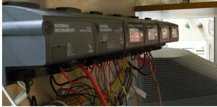
Figure 3-7 Field-point used as an interface of the electronic devices and LabVIEW program.
