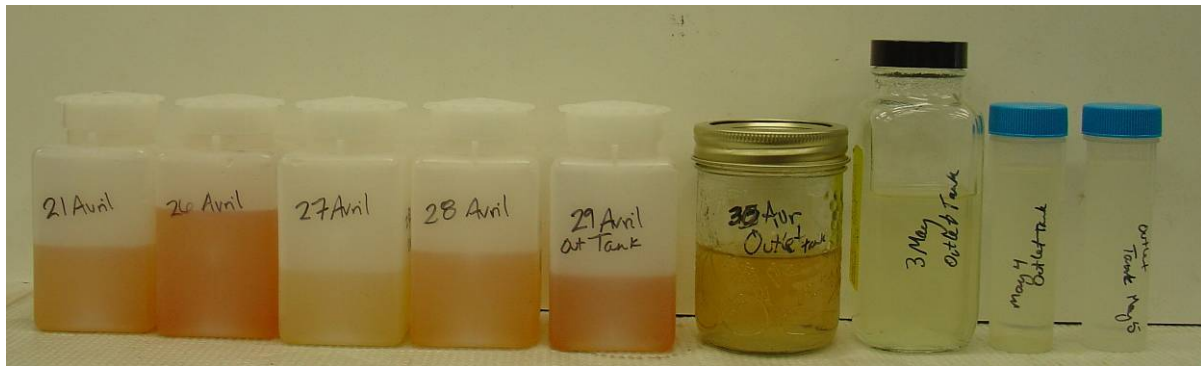
Figure 6.27 Loading test: Biofilter outlet solution, orange left: day 6-15, clear right: day 18-20
