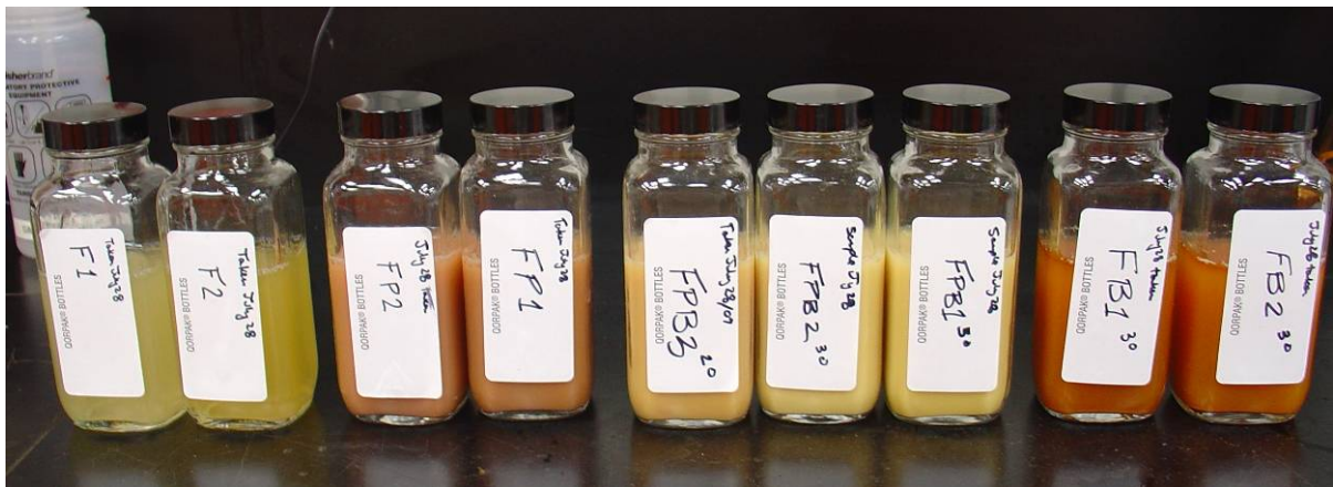
Figure 6.3 Packing test solutions at media change - Agitated, day 20 (grown at 150rpm, 25°C)
