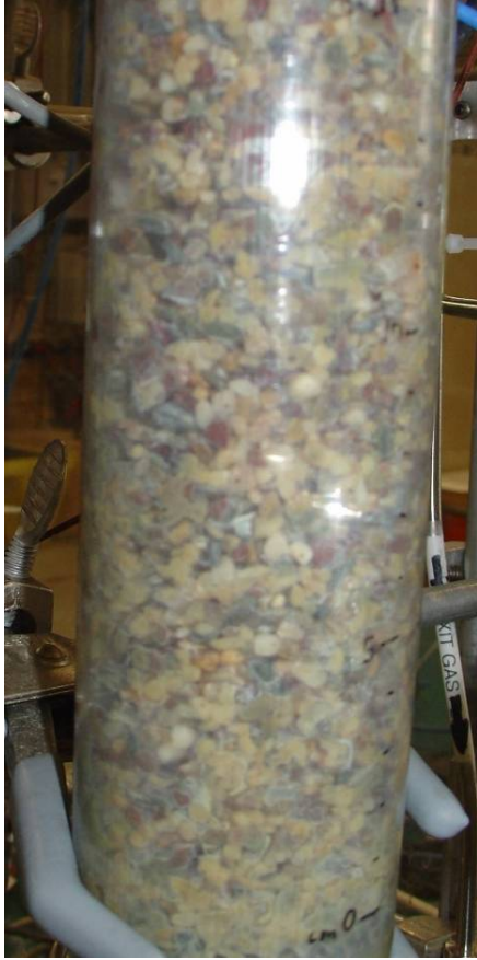
Figure 6.25 Biofilter packed bed: Startup and acclimatization, day 7
