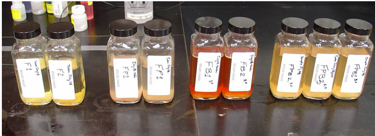
Figure 6.4 Packing test solutions at media change – Settled, day 20 (grown at 150rpm, 25°C)
