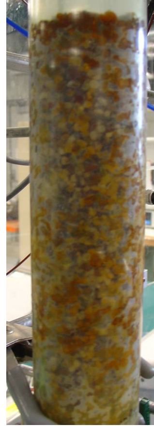
Figure 6.26 Biofilter packed bed: Startup and acclimatization, day 21
