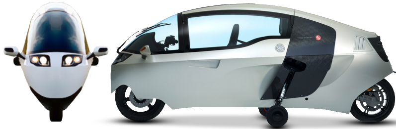
Fig.2.3 MonoTracer: closed-cockpit, two-seater, motorcycle with automated stabilizers
