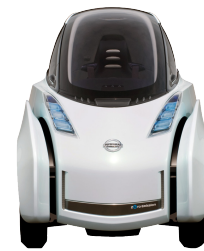
Fig.2.6 Land Glider: electric, tilting, two-seater microcar
