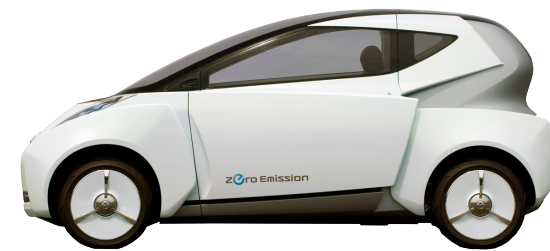
Fig.2.6 Land Glider: electric, tilting, two-seater microcar
