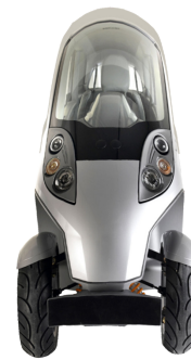
Fig.2.7 Lumeneo: fixed-axel, low-speed, electric, two-seater microcar
