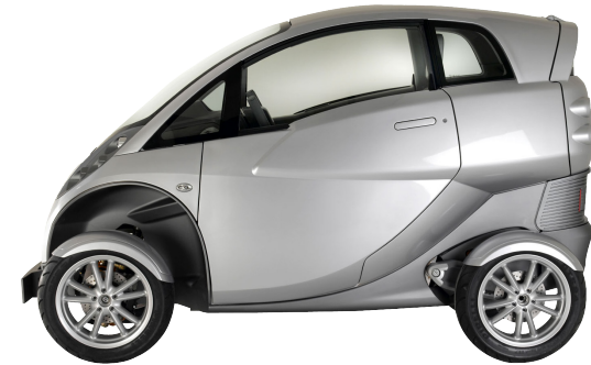
Fig.2.7 Lumeneo: fixed-axel, low-speed, electric, two-seater microcar
