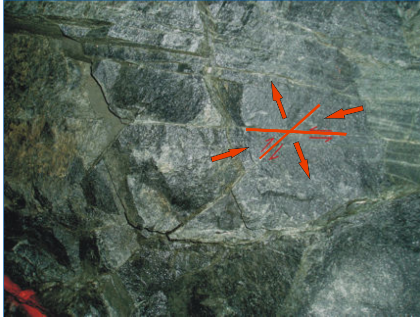
Figure 12. Photograph showing the mutually overprinting relationship and opposing senses of slip along conjugate fracture planes in the Tanco mine.
