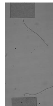
(c) Released 2\mu\text{m} clamped-clamped beam, broken.
