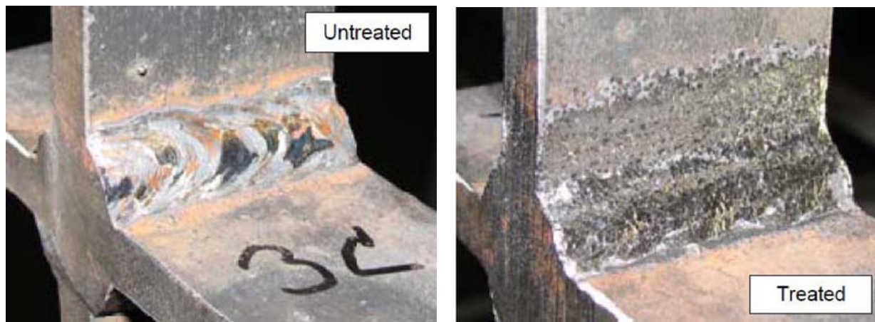
Figure 3.9: Fatigue specimen weld toe; Left: untreated, Right needle peened (photo: [Walker et al. 2008])
