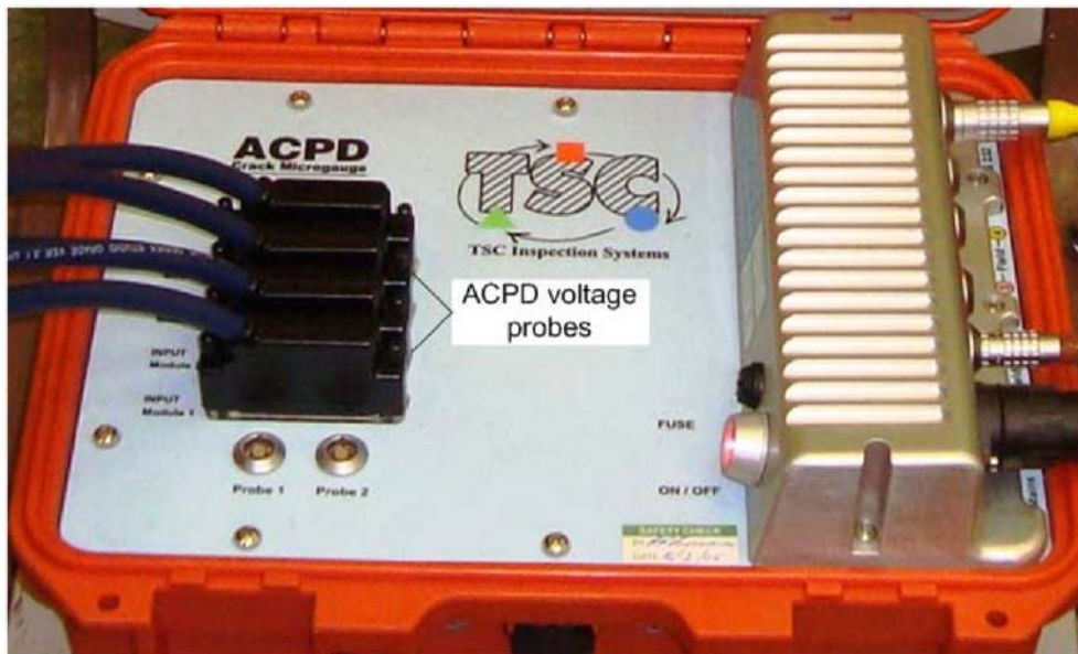
Figure 3.12: ACPD measurements tools; ACPD probes attached to the specimen (top); Acquisition box (bottom)
