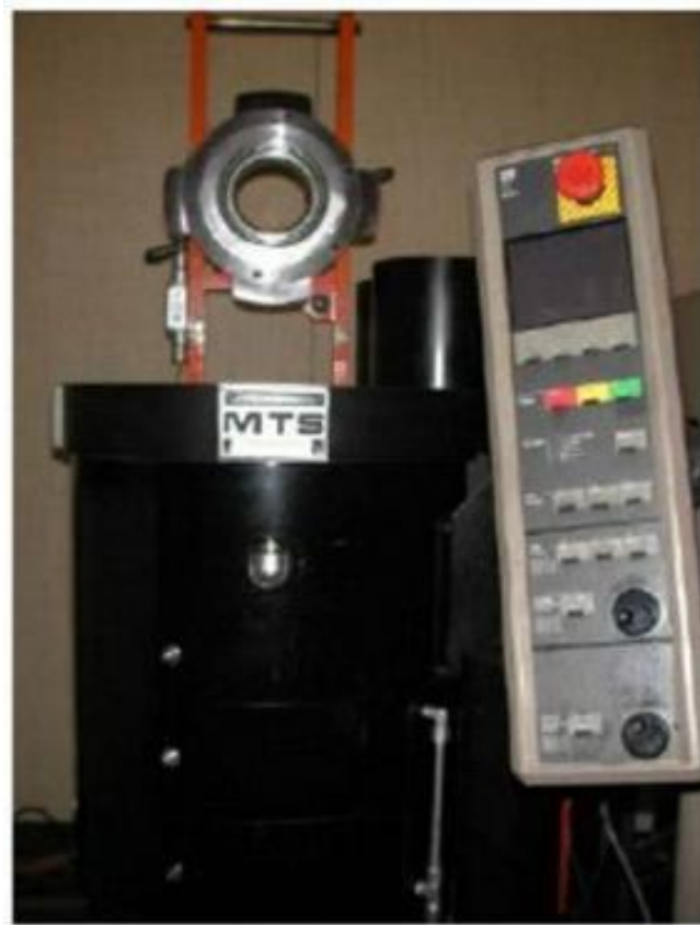
Figure 3.12 MTS 866.02 formability press [79]
