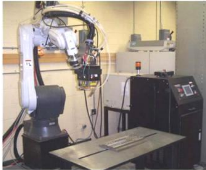
Figure 3.6 Nuvonyx diode laser head mounted on a Panasonic robotic arm
