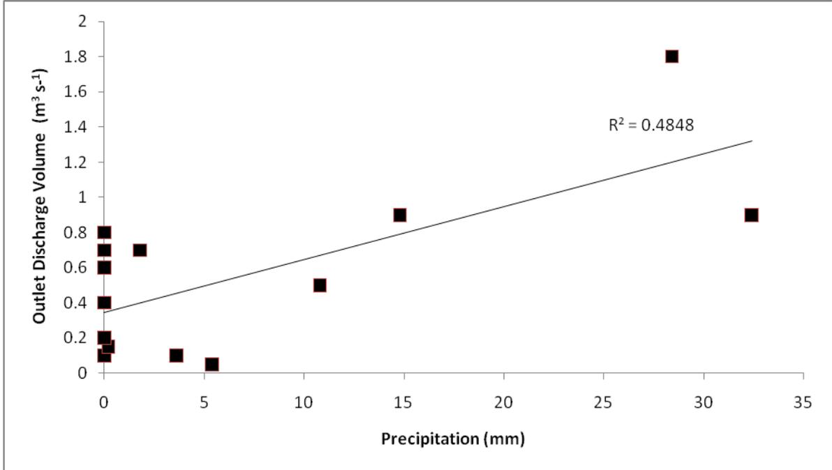
Figure 3b: The relationship between precipitation and outflow water volume (discharge) for Columbia Lake outflow in 2007, calculated from area velocity method by H. Yu 2007.
