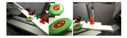
Figure 6.16: Experiment 4: Effect of lens distortion on the appearance of objects. The  $(\alpha, \beta)$  angles of the camera are  $(-25^{\circ}, -40^{\circ})$  for the left image and  $(35^{\circ}, -53^{\circ})$  for the right image. The values of  $(r, \theta, \phi)$  are the same for both cases. The non-affine stretching of the green toy in the right image makes it difficult to identify during the visual search
