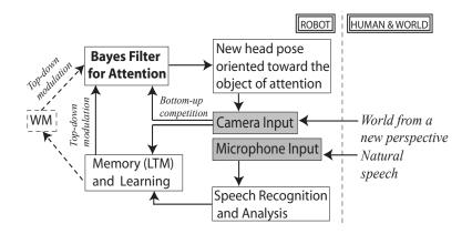
Figure 5.1: Functional description of the proposed model. Visual search and visual exploration is integrated through robot learning and speech-based interaction with the human
