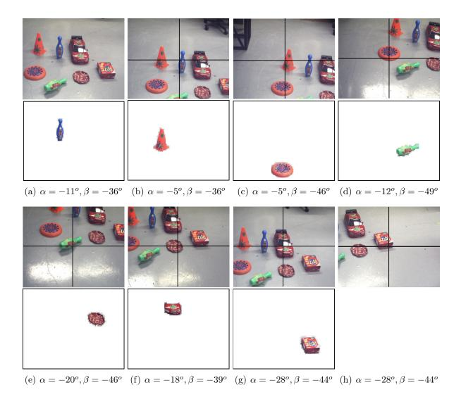
Figure 4.3: Different stages of the visual exploration experiment shown in Fig. 4.2. For each image the top row indicates the frame captured at the beginning of a decision cycle and the bottom row indicates the objects to be focused at the successive decision cycle based on the estimated head-pose  $(\alpha, \beta)$  shown within parenthesis. After attending the object in (h), the robot can not identify any other novel stimulus in the VF and remains at the current state
