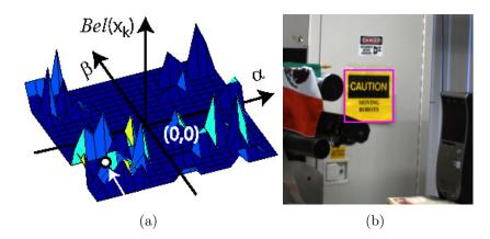
Figure 3.8: (a) The weighted samples representing the posterior for attention. The particle with highest weight (marked by the white circle) is reported as the next head-pose of the robot (b) The object (marked by a rectangle) focused at the new head-pose (please see text for detail)
