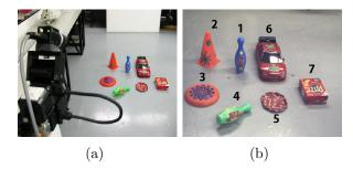
Figure 4.2: Novelty-guided visual exploration with relative proximity-based analysis (a) The experimental environment with seven novel objects (b) The VF of the robot at the first decision cycle. In the successive cycles the objects are attended in order of their proximity to the current focus of attention. The numbers denote the sequence of attention (please see text and Fig. 4.3 for detail)
