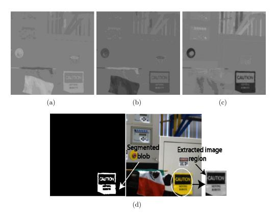
Figure 3.6: Object segmentation process corresponding to the image in Fig. 3.5(a). The images after the pyramid-based image segmentation (a)  $I_k^{\rm r'}$  (b)  $I_k^{\rm g'}$  (c)  $I_k^{\rm b'}$  (d) The segmented object blob corresponding to the head-pose ( $\alpha = -9^o, \beta = -20^o$ ) and the image region considered for SIFT keypoint extraction based on the bounding rectangle of the segmented blob
