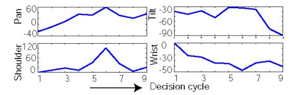
Figure 6.15: Experiment 4: Positions of the camera, shoulder and the wrist joint during the experiment. The shoulder and wrist angles are with respect to the world coordinate system
