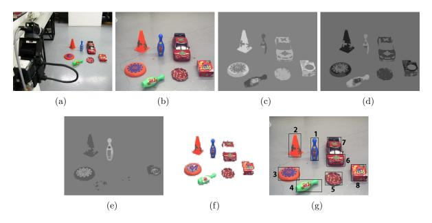
Figure 4.17: Effect of the image processing parameters: visual exploration experiment with  $\zeta_1 = 24$  and  $\zeta_2 = 20$ . (a) The experimental environment (b) The visual field of the robot at the first decision cycle. (c)-(e) The images  $I^{r'}, I^{g'}$  and  $I^{g'}$  corresponding to the visual field (f) The object blobs segmented from the image in (a) during the visual exploration experiment. (g) The attention sequence of the robot during the experiment (please see text for detail)
