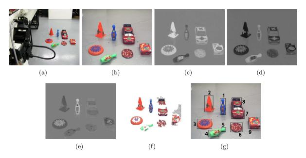
Figure 4.16: Effect of the image processing parameters: visual exploration experiment with  $\zeta_1 = 6, \zeta_2 = 5$ . (a) The experimental environment. (b) The VF of the robot at the first decision cycle. (c)-(e) The images  $I^{r'}, I^{g'}$  and  $I^{g'}$  corresponding to the VF. (f) The object blobs segmented from the image in (a) during the visual exploration experiment. (g) The attention sequence of the robot during the experiment (please see text for detail)
