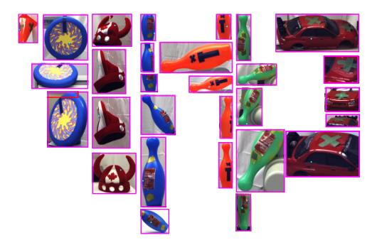
Figure 6.9: Experiment 3: On-spot learning. Different views of the objects chosen by the robot to learn. The SIFT keypoints corresponding to these views are stored in the LTM
