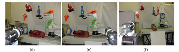
Figure 6.8: Experiment 3: The robot is exposed to a set of objects from different 3D locations in the world and learns about them while being guided by its continuously developing sense of novelty. The camera locations  $(r, \theta, \phi, \alpha, \beta)$  are (a)  $(6ft, 85^o, 50^o, -5^o, 0^o)$  (b)  $(6.5ft, 68^o, 52^o, 15^o, 5^o)$  (c)  $(6.5ft, 68^o, 52^o, -15^o, 5^o)$  (d)  $(3ft, 75^o, 30^o, -5^o, 0^o)$  (e)  $(3ft, 80^o, 30^o, 8^o, 5^o)$  (f)  $(6.5ft, 68^o, 52^o, -15^o, 5^o)$
