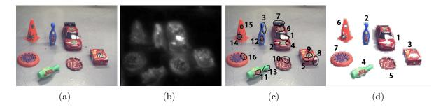
Figure 4.5: Novelty guided visual exploration with relative saliency-based analysis (a) The visual field of the robot at the first decision cycle where all seven novel objects are visible. (b) The saliency map of the visual field generated using the VOCUS algorithm [23]. (c) The first sixteen focuses of attention suggested by the saliency map. (d) The first seven objects of attention evaluated according to the modified VOCUS algorithm (please see text for detail)
