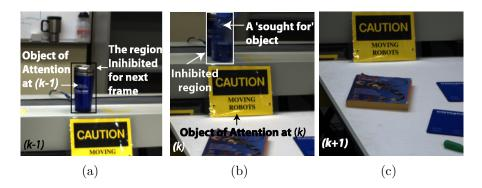
Figure 1.6: Difficulty in visual search with space-based dynamic IOR (a) The region of the attended object at time (k - 1) is made inhibited for time k, (b) The inhibited region is mapped to the new image coordinate system at time k. A 'sought for' object appears within the inhibited region and the robot ignores its presence, (c) A random head movement in search of the 'sought for' object causes it to go out of the VF. As a result, the robot requires longer time to find the 'sough for' object
