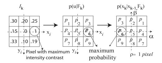
Figure 3.3: Evaluation of the bottom-up competition model for a hypothetical  $3 \times 3$  camera image. The numbers in  $I_k$  represent the intensity values of different pixels and  $p_1, \ldots, p_9$  indicate their probabilities. Here,  $\rho = 1$  (please see text for detail)
