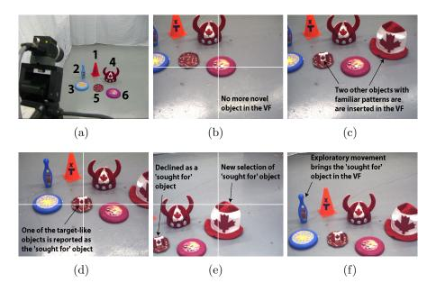
Figure 6.4: Experiment 2A: Integration of visual exploration and visual search (a) The experimental environment with several novel objects. The numbers denote the sequence at which different objects are attended (b)-(f) The visual fields of the robot at different stages of the experiment (please see text and the attached multimedia file "Multimedia\_Generality.wmv" for detail)
