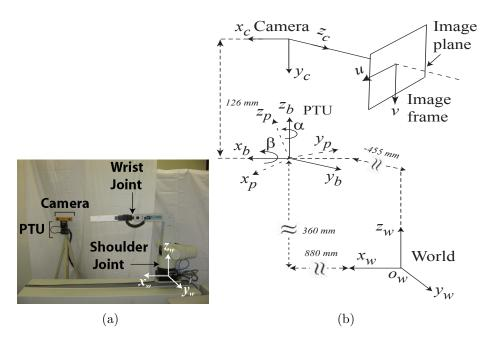
Figure 5.2: (a) The experimental set-up: the robotic manipulator used for pointing behavior, the PTU and the camera (b) The coordinate systems involved with the setup
