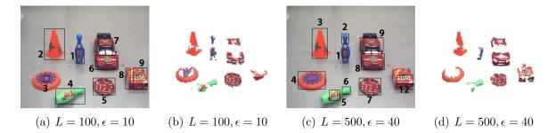
Figure 4.15: The effect of the block size on the visual attention behavior. The attention sequences resulted from using different combinations of values for  $\epsilon$  and L are marked on the first VF of the robot and shown in (a) and (c). The segmented object blobs are shown in (b) and (d) (please see text for detail)
