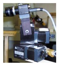
Figure 4.1: A Point Grey Research Flea2 color camera mounted on a Directed Perception PTU constitutes a robotic camera-head and is used during the experiments
