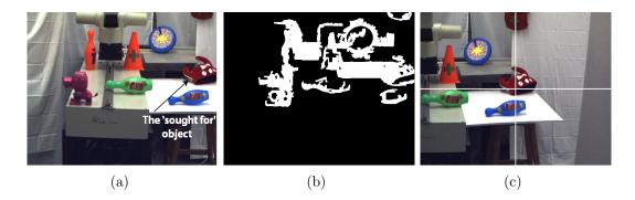
Figure 6.11: Experiment 3 (a) The visual field where the *red hat* is searched (b) Incorrect region growing causes the the *red hat* to become a part of the large object blob which is discarded from further analysis of attention due to its large size (c) The *red hat* is focused
