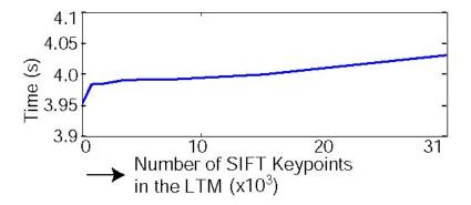
Figure 4.20: Time required to identify a novel object with varying memory (LTM) sizes (corresponding to the experiments demonstrated in Fig. 4.19)
