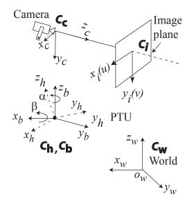
Figure 1.5: The coordinate systems involved with robotic overt visual attention for a simple camera-PTU arrangement (please see text for detail)
