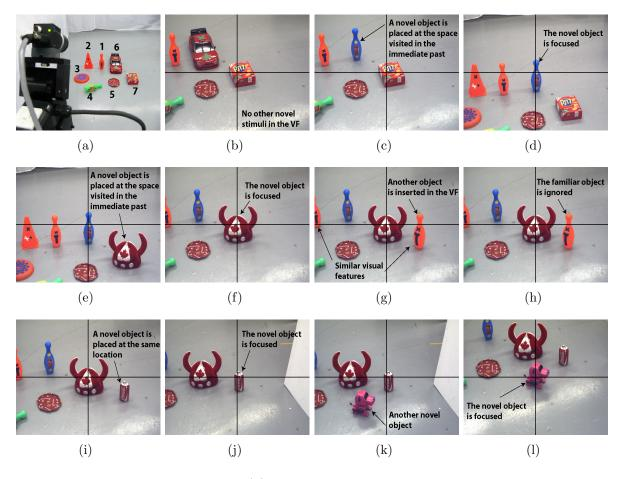
Figure 4.9: Demonstration of IOR: (a) The experimental environment and the sequence of attention. (b)-(j) Different stages of the experiment (please see the text and the multimedia file "Multimedia\_IOR.wmv" for detail)
