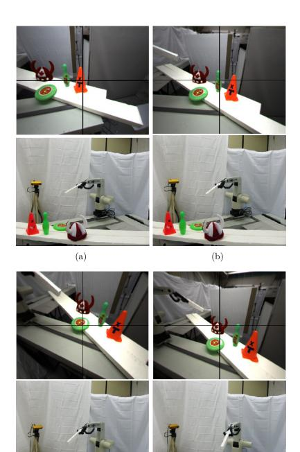
Figure 6.14: Experiment 4: in each case the top image shows the camera focusing on an object (due to its novelty or search request for it) and the bottom image show the manipulator pointing to the focused object to make it more salient to the human operator (please see text and the attached multimedia file "Multimedia\_AttentionAndPointing.wmv" for detail)
