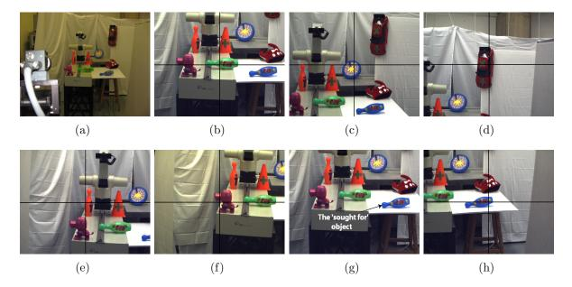
Figure 6.10: Experiment 3: on-spot learning. (a) The experimental environment. (b)-(f) Focusing on different 'sought for' objects: green pin, blue toy, red car, orange pin, and purple dog. (g) Failure to identify the blue pin due to large change in orientation. (h) The blue pin is focused through on-spot learning (please see text and the attached multimedia file "Multimedia\_On-SpotLearning.wmv" for detail)
