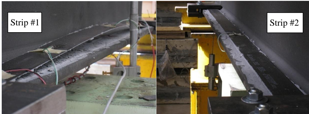
Figure 4.27. Debonding of strips for specimen 15%-F-S
