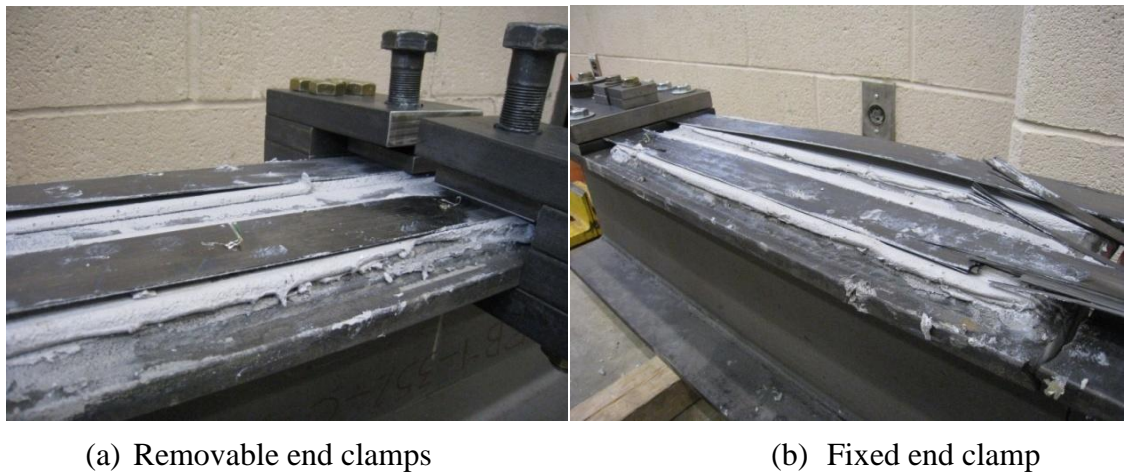
Figure 4.32. Performance of end clamps after failure for specimen 37%-C-M
