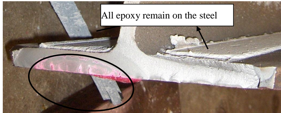
Figure 4.25. Elliptical crack growth pattern through the thickness of flange and interfacial debonding between epoxy and strips (specimen 14%-F-M)
