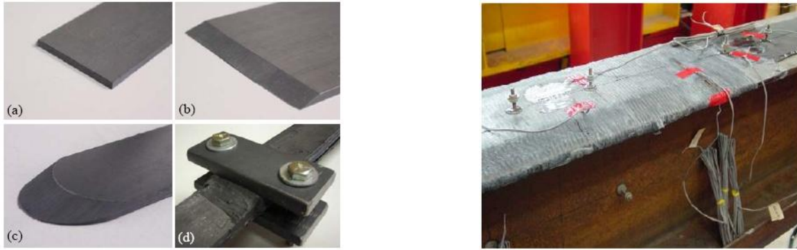
(c) (1) square, (2) tapered, (3) rounded and (4) clamped plate ends.
