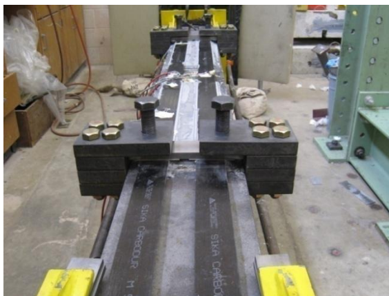
(a) Completed prestressing system for the strips on the cover plates.
