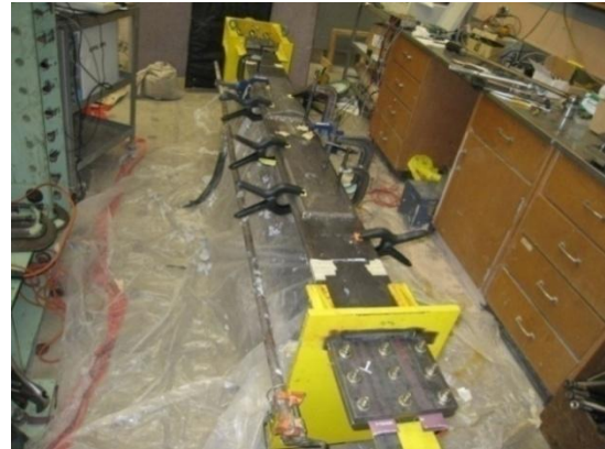
(b) Clamped strips to the beam after prestressing
