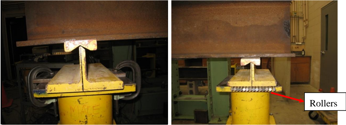
(b) Simple support (c) Roller support Figure 3.22. Test setup and support configurations
