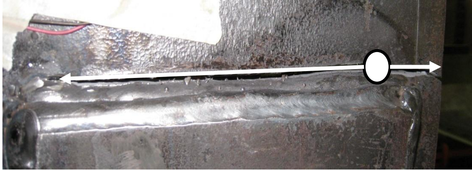
Figure 4.22. Crack initiation and propagation along the weld for control specimen
