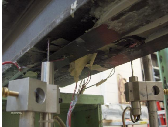
Figure 3.24. LVDTs at the midspan during fatigue tests
