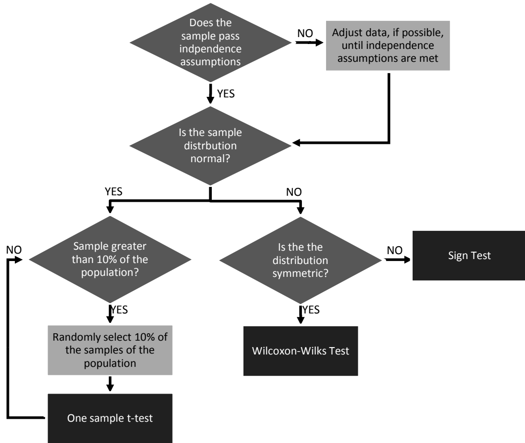
Figure A-2: Process taken to determine the application of which statistical test
