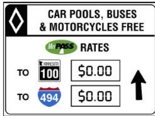
Figure 2.5: Example of an I-394 MnPASS sign displaying the posted toll rate Source: Halvorson et al. (2006)
