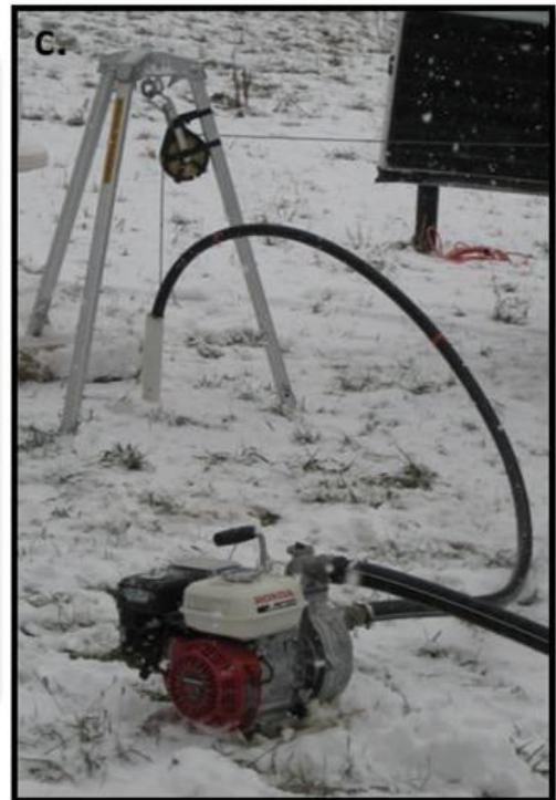
Figure 3.5: (a) The impeller flowmeter used for borehole logging. (b) The Mount Sopris 4MXA-1000 winch used to control the measurement depths. (c) The surface instrumentation, including the tri-pod and pulley system used to suspend the instrument and the Honda WH15XK1C1 high-pressure pump.
