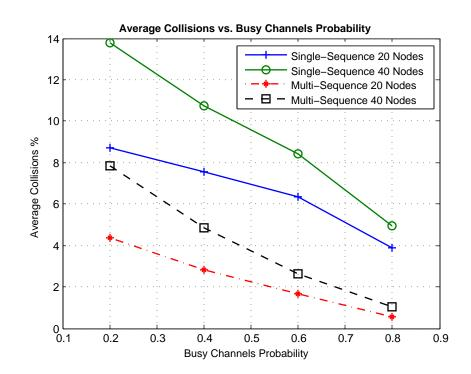
Figure 3.24: PU Collision percentage versus Busy Channel Probability
