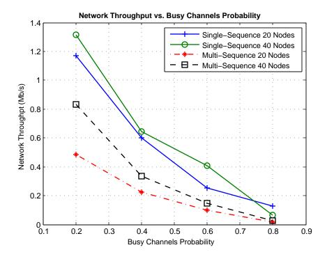
Figure 3.23: Network Throughput versus Busy Channel Probability
