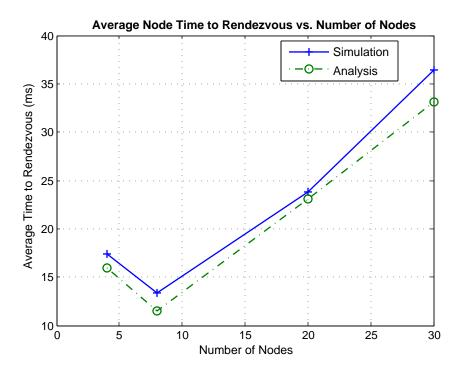
Figure 3.15: Average TTR for Simulation and Analysis versus Number of Nodes
