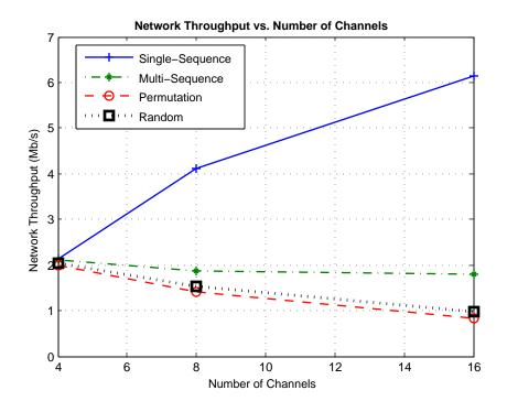
Figure 3.20: Protocols Throughput versus Number of Channels
