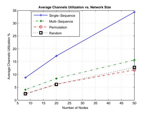
Figure 3.19: Average Channels Utilization Comparison versus Number of Nodes
