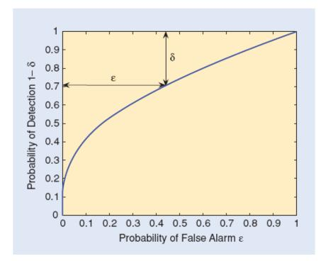
Figure 2.1: False Alarm versus Detection Probabilities [2]
