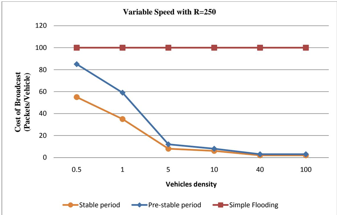
Figure 6: First scenario (variable speed, broadcasting cost vs. density)
