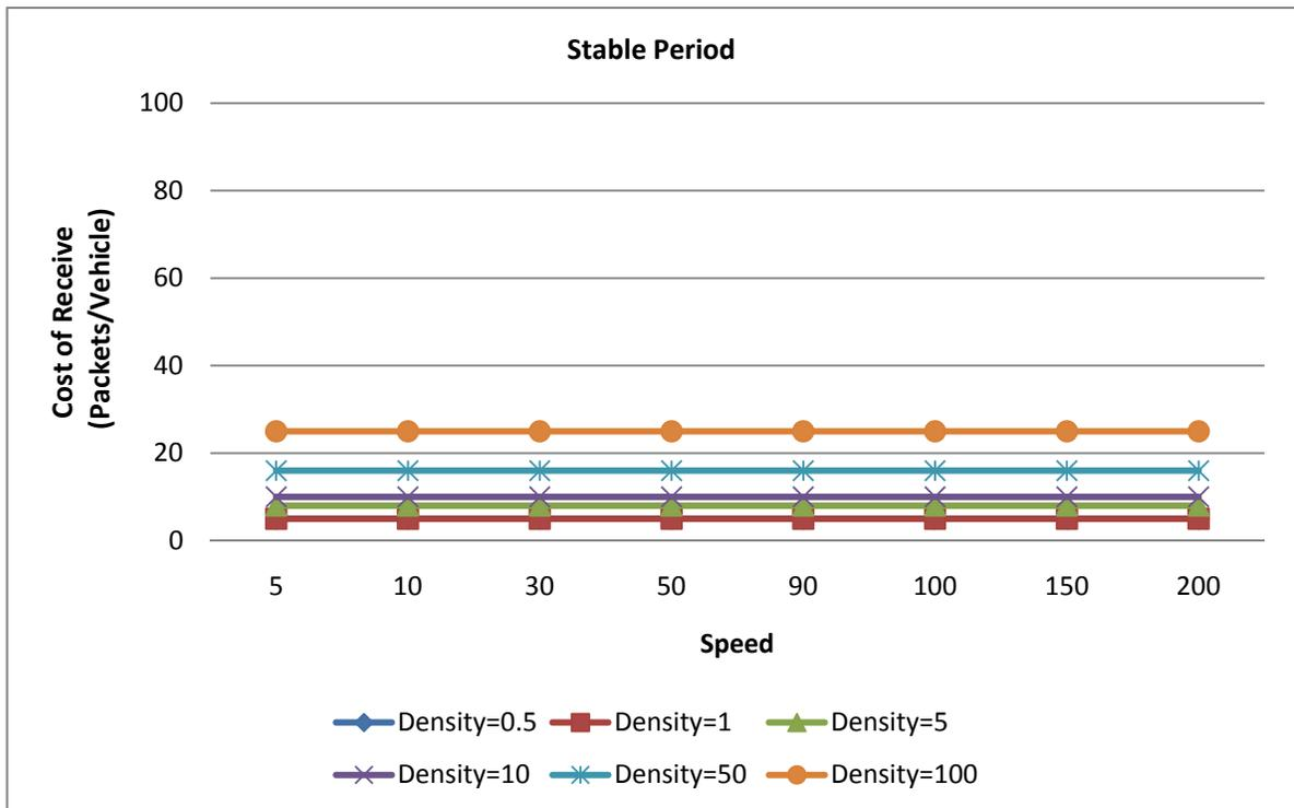
Figure 13: Second scenario (stable period, receiving cost vs. speed)
