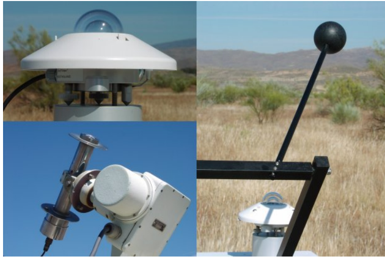
Figure 2-2 Pyranometer (left top), Two-axis tracked Pyrheliometer (left bottom), Pyranometer with shading ball (right)
