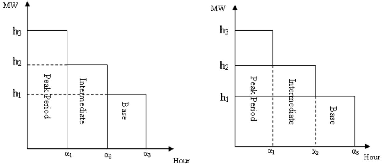
**Figure 4-4: Vertical and Horizontal Approximation of Annual Load Duration Curve**
