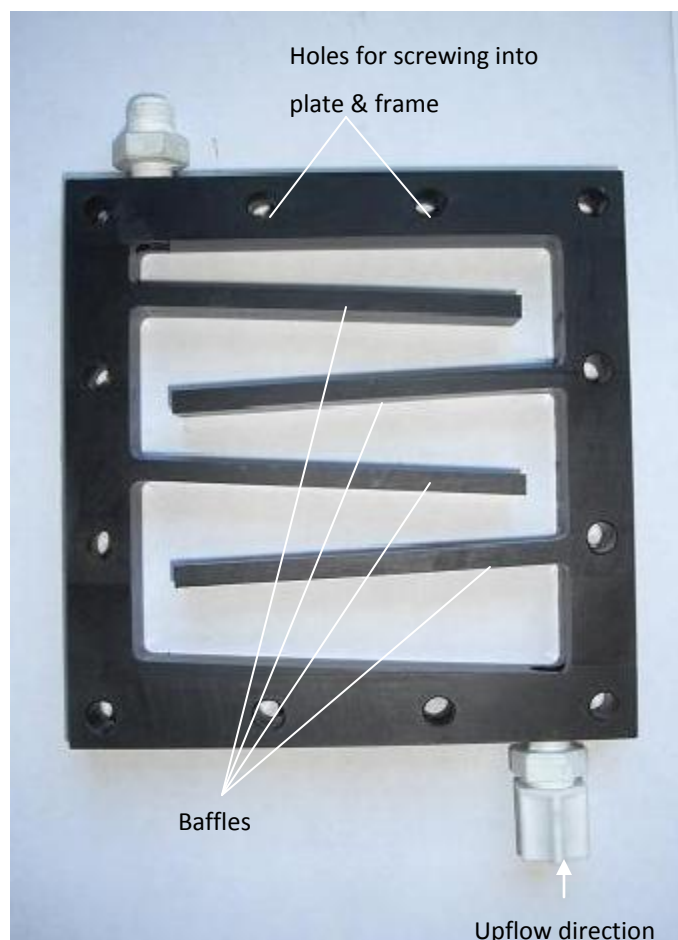
Figure 4.1 Baffled analyte chamber of MFC
