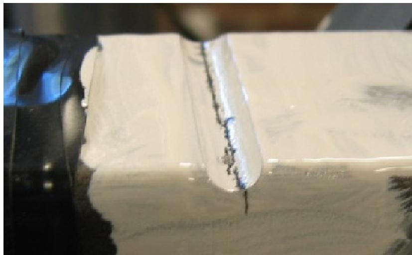
Figure 94. Notched sample with an obvious edge crack.
