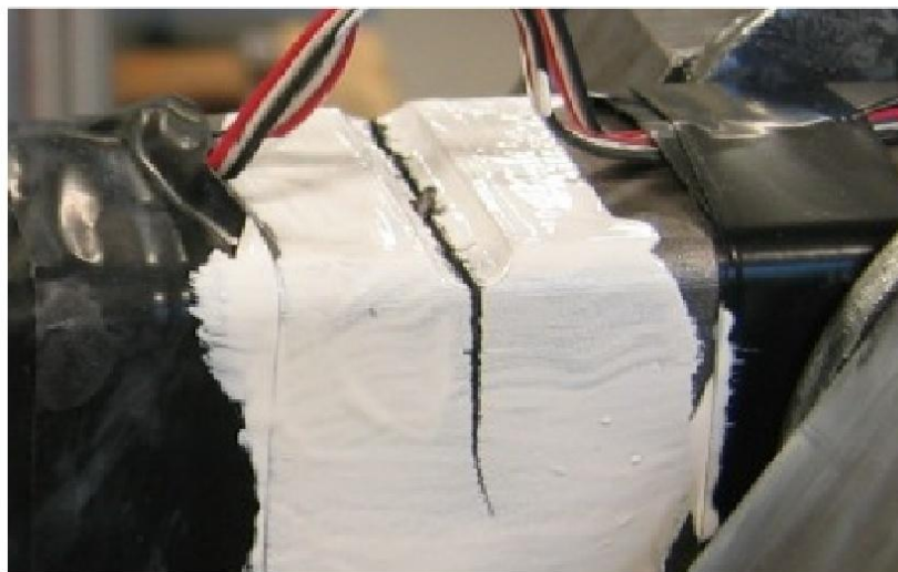
Figure 95. Failure in the notched sample.
