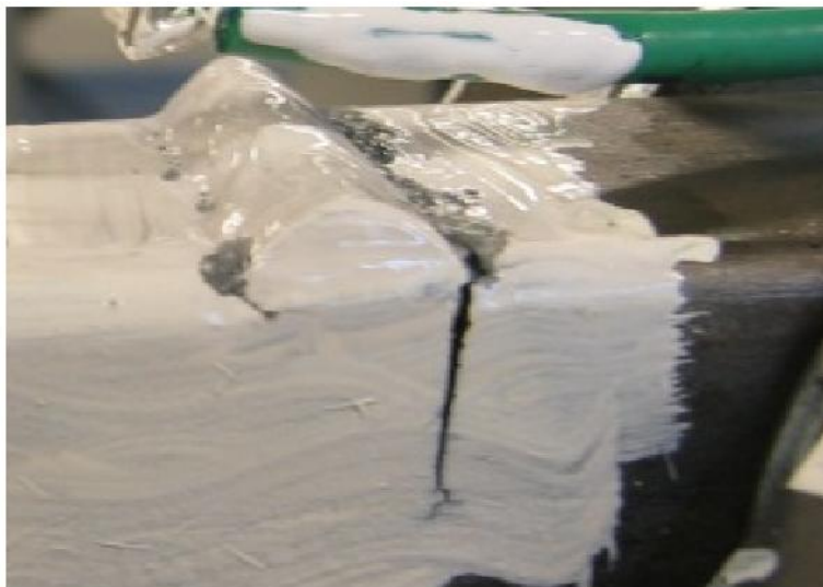
Figure 108. Final failure of the welded component.
