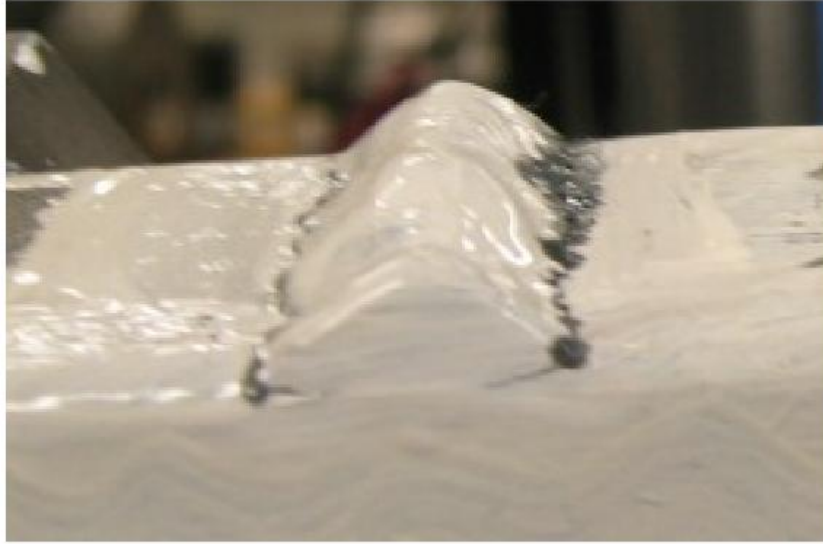
Figure 106. Crack across the width of the weldment.
