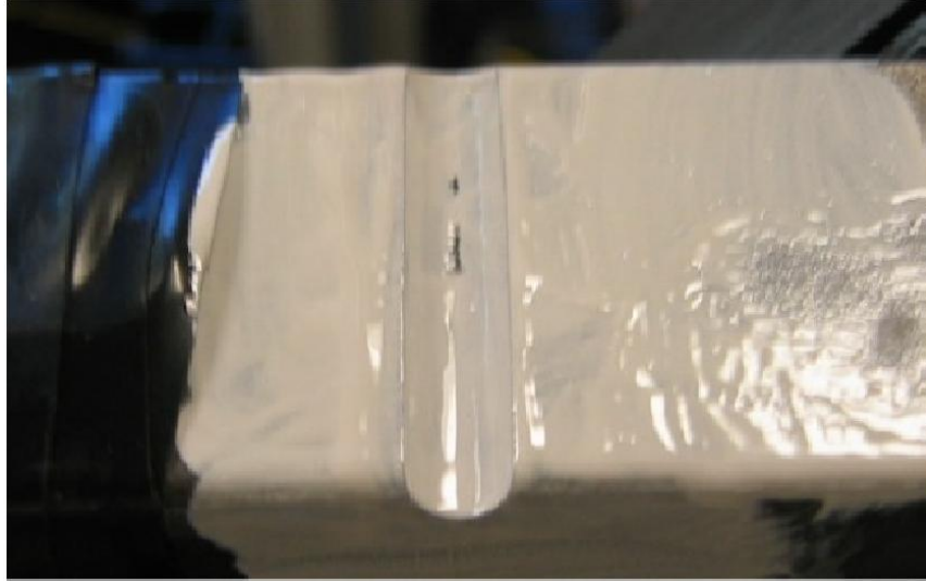
Figure 90. Notched sample crack initiation
