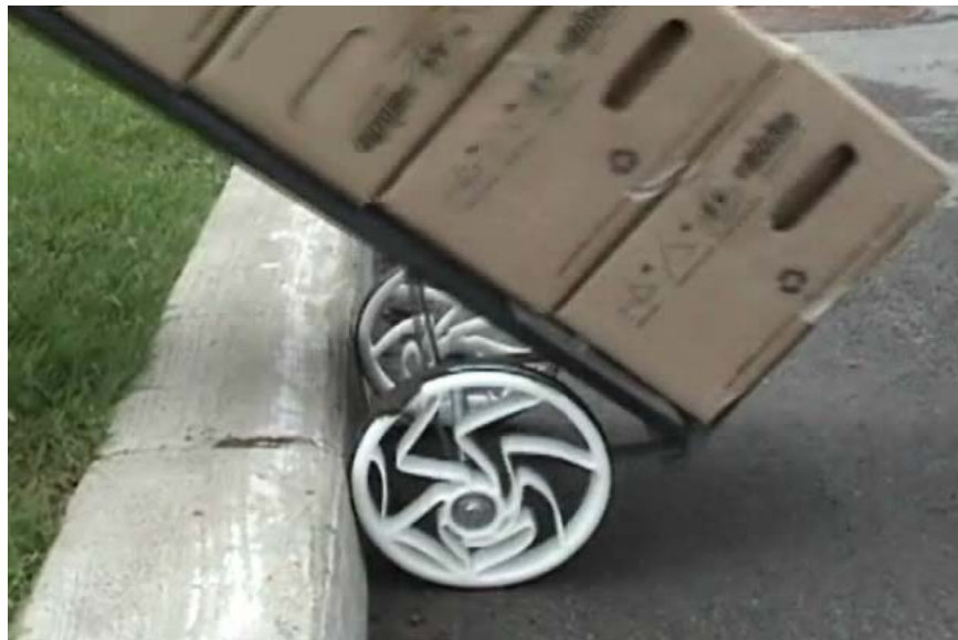
Figure 5.3 - The prototype installed on a hand truck
