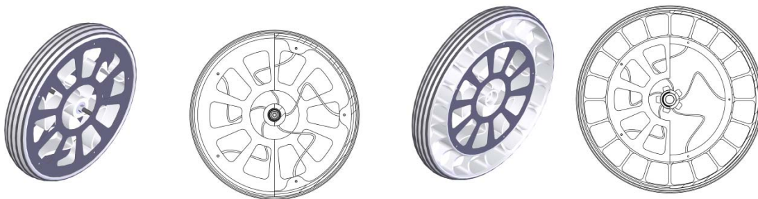
Figure 5.5 - Fixed joint IWS design for baby stroller; Left: front wheel Right: rear wheel
