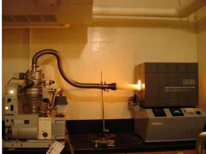
Figure 3.2 The apparatus of vacuum oven used for the vacuum brazing of CNTs strands.
