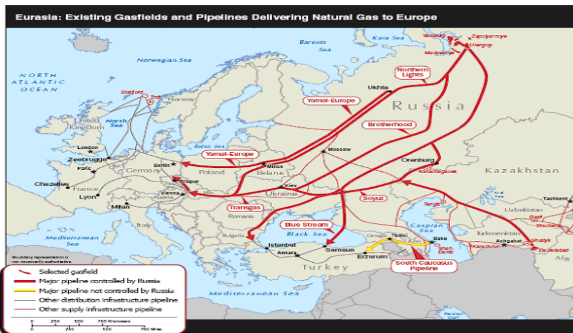
Figure 1.1 European and Eurasian Natural Gas Infrastructure 8
