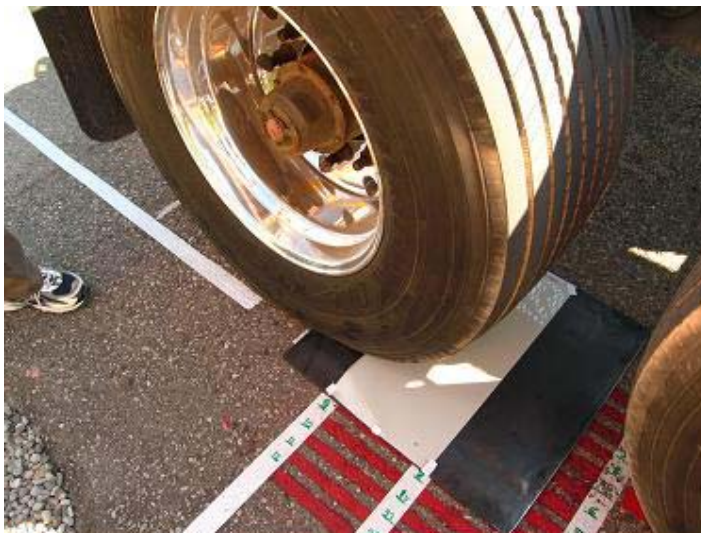
Figure 3-10: Pressure Sensor Pad used to Measure Tire Contact Pressure
