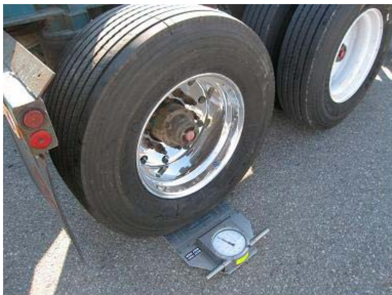
Figure 3-8: Mobile Scale Used to Verify Single Axle Loads
