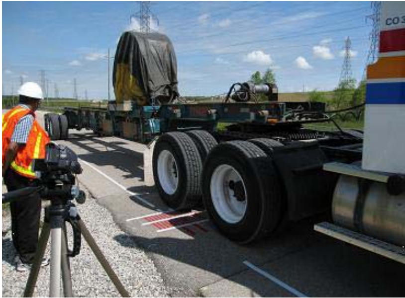
Figure 3-9: Camera and Pavement Markings Used to Verify Wheel Load Location over ASG1 and ASG5
