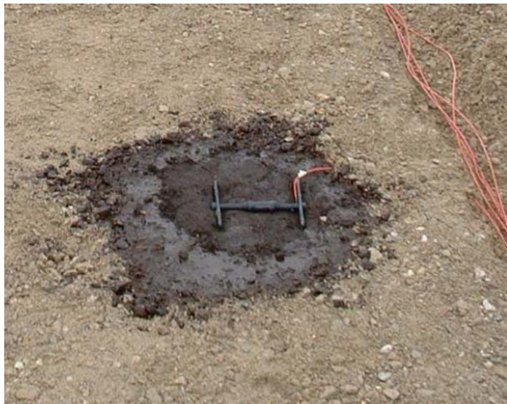
Figure 3-3: H-type Asphalt Strain Gauge Prior to Placement of HL3 Asphalt (Adedapo 2007)
